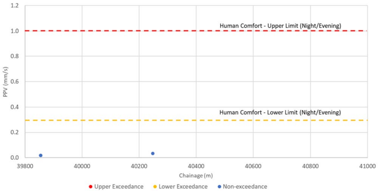
FIGURE 15.3: PREDICTED ROADHEADER PEAK PARTICLE VELOCITY (MM/S) AT SENSITIVE RECEPTORS ALONG THE TUNNEL ALIGNMENT AND THE TRANSPORT NOISE MANAGEMENT CODE OF PRACTICE: VOLUME 2—CONSTRUCTION NOISE AND VIBRATION HUMAN COMFORT VIBRATION CRITERIA
