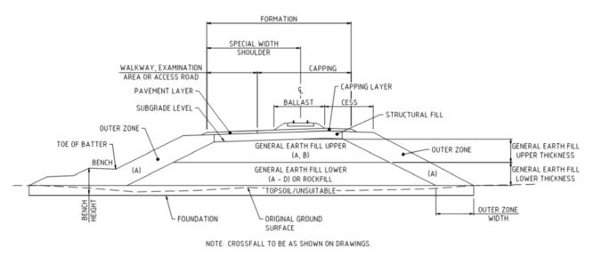
FIGURE 2.2: SCHEMATIC OF ZONED EMBANKMENT CROSS SECTION
