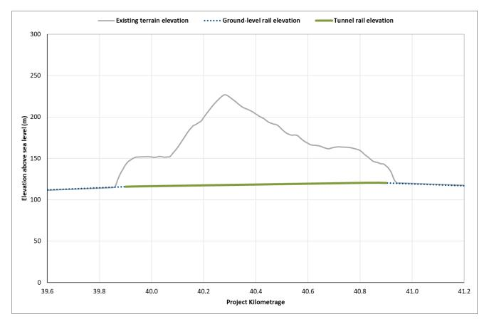
The single-track is to be located close to the centre of the tunnel to deliver the internal space necessary to facilitate the ventilation requirements. At the extents of the tunnel, tunnel portals shall be excavated to facilitate the transition between the ballasted surface track and the slab track within the tunnel structure.
