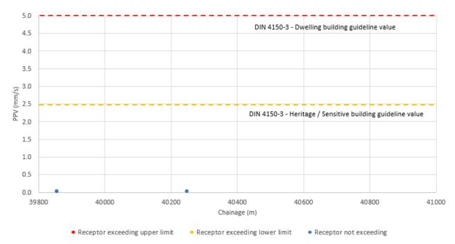
Figure 5.2 Predicted roadheader PPV (mm/s) at the sensitive receptors along the tunnel alignment and the long-term DIN 4150-3 damage guideline values
