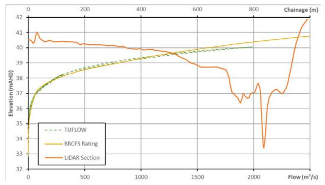
Figure 7.4 Comparison of TUFLOW flow-depth relationship with Rosewood rating
