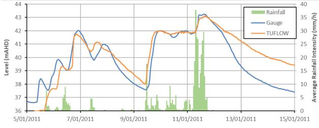
Figure 7.10 Comparison of TUFLOW and recorded water levels at Rosewood WWTP for the 2011 flood
