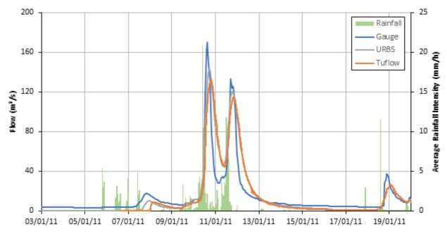
Figure 7.28 Comparison of URBS, TUFLOW and stream gauge hydrographs at Peak Crossing for the 2011 event
