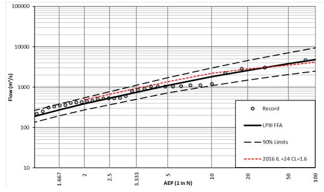
Figure 8.5 Flood frequency analysis – Yarrahapinni gauge
