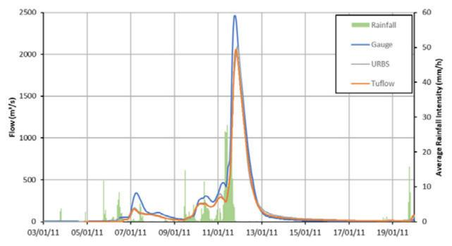
Figure 7.11 Comparison of URBS, TUFLOW and stream gauge hydrographs at Walloon for the 2011 flood
