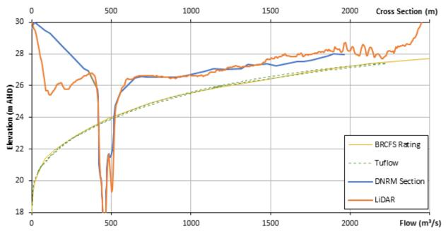
Figure 7.3 Comparison of TUFLOW flow-depth relationship with Walloon rating
