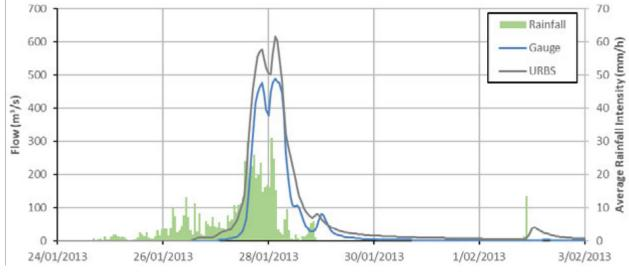
Figure 7.13 Comparison of URBS and stream gauge hydrographs at Adam's Bridge for the 2013 flood
