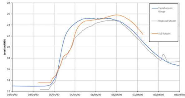
Figure 7.36 Comparison of Regional, Sub-model TUFLOW and stream gauge flood levels at Yarrahapinni for the 1990 event
