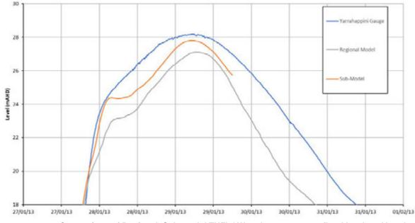
Figure 7.37 Comparison of Regional, Sub-model TUFLOW and stream gauge flood levels at Yarrahapinni for the 2013 event
