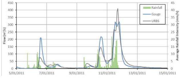
Figure 7.9 Comparison of URBS and stream gauge hydrographs at Adam's Bridge for the 2011 flood
