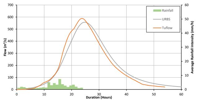
Figure 8.8 Comparison of URBS and TUFLOW hydrographs at Loamside for 1% AEP flood event
