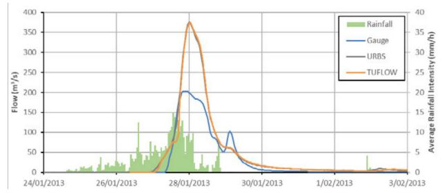
Figure 7.14 Comparison of URBS, TUFLOW and stream gauge hydrographs at Kuss Road for the 2013 flood
