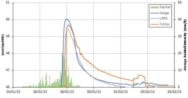
Figure 7.30 Comparison of URBS, TUFLOW and stream gauge flood levels at Peak Crossing for the 2013 event
