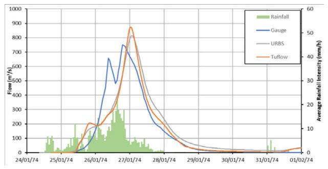
Figure 7.25 Comparison of URBS, TUFLOW and stream gauge hydrographs at Loamside for the 1974 event
