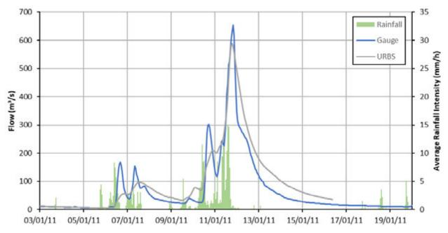
Figure 7.20 Comparison of URBS and stream gauge hydrographs at Junction Weir for the 2011 event
