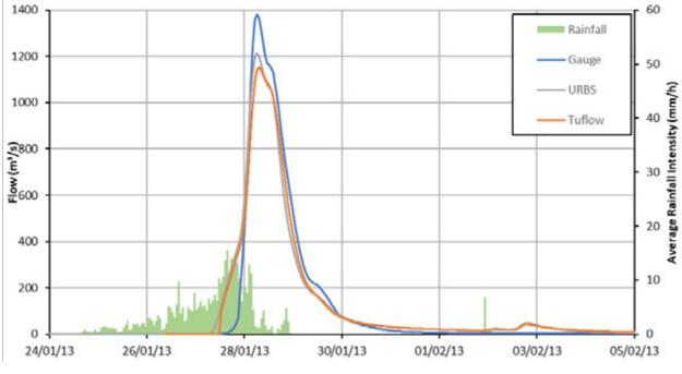
Figure 7.15 Comparison of URBS, TUFLOW and stream gauge hydrographs at Walloon for the 2013 flood
