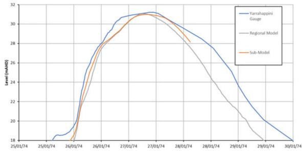
Figure 7.35 Comparison of Regional, Sub-model TUFLOW and stream gauge flood levels at Yarrahapinni for the 1974 event
