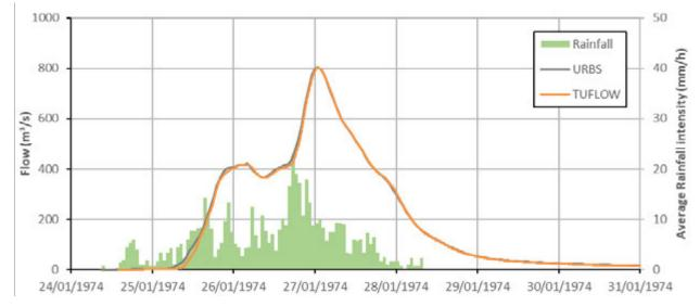
Figure 7.7 Comparison of URBS and TUFLOW hydrographs at Kuss Road for the 1974 event
