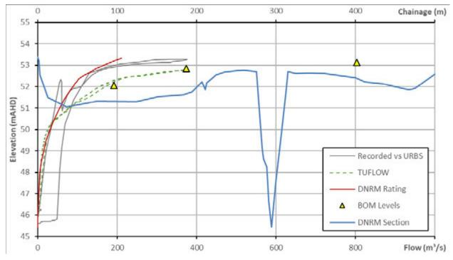
Figure 7.5 Comparison of TUFLOW flow-depth relationship with Kuss Road rating
