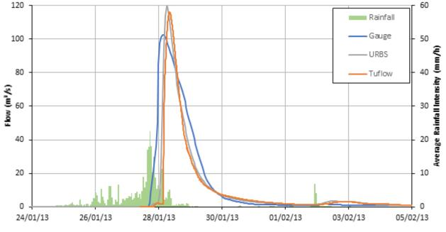
Figure 7.29 Comparison of URBS, TUFLOW and stream gauge hydrographs at Loamside for the 2013 event
