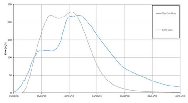
Figure 7.32 Comparison of RAFTS and Gauge hydrographs at Overflow for the 1990 event
