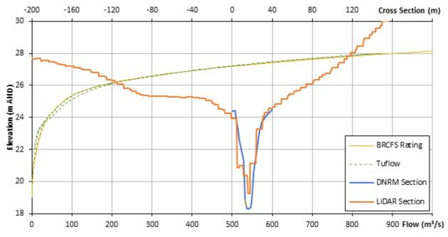
Figure 7.23 Comparison of TUFLOW flow-depth relationship with Loamside rating
