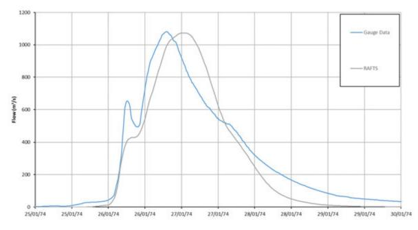
Figure 7.31 Comparison of RAFTS and Gauge hydrographs at Overflow for the 1974 event
