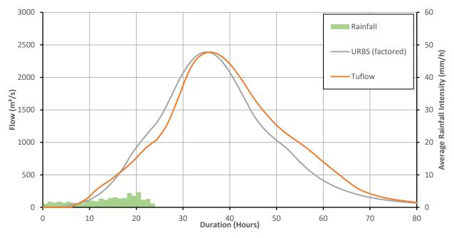
Figure 8.7 Comparison of URBS and TUFLOW hydrographs at Amberley for 1 % AEP flood event (factored flow, no dams)
