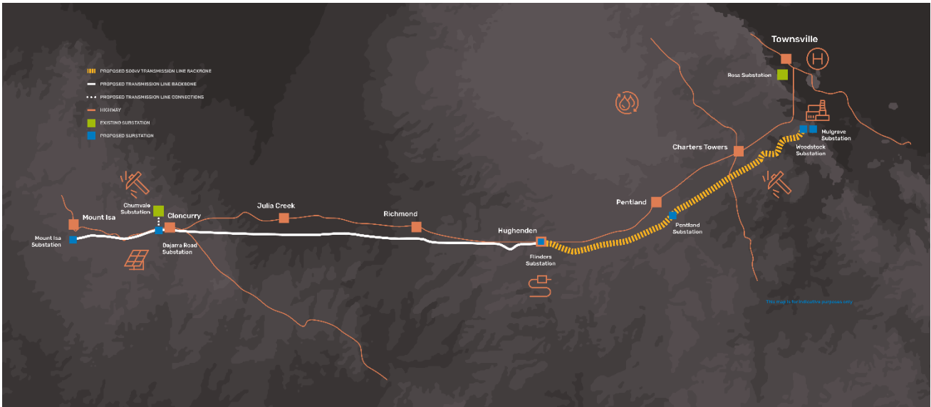
Figure 22: CopperString 2032 proposed transmission lines and substations
