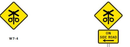
Figure 30: Railway crossing ahead active control signs
