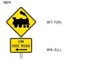
Figure 26: Railway crossing ahead passive control signs – on side road
