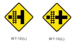
Figure 27: Railway crossing diagrammatic warning assemblies – on side road
