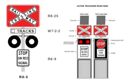
Figure 29: Railway crossing flashing signal assembly
