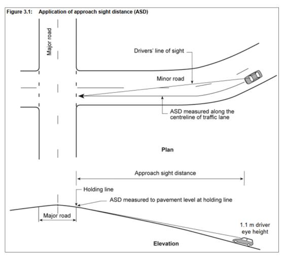
Figure 15: Austroads Guide to Road Design Part 4A: unsignalised and signalised intersections application of ASD
