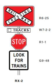
Figure 23: Railway crossing stop assembly (RX-2)
