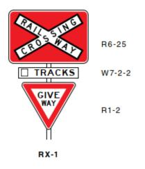
Figure 22: Railway crossing give-way assembly (RX-1)
