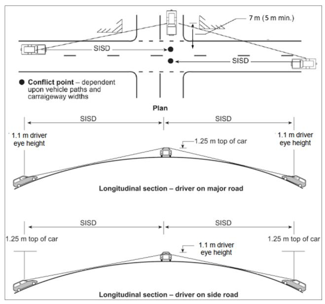
Figure 17: Supplement to AGRD Part 4A SISD
