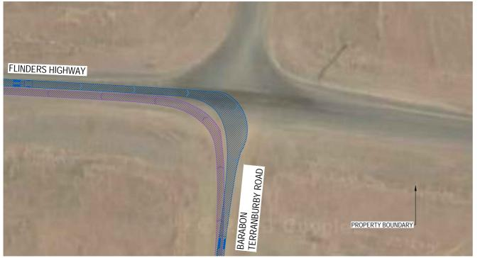
26m B-DOUBLE ENTERING WEST 8.8m SERVICE VEHICLE EXITING WEST SCALE 1:500 (m)
