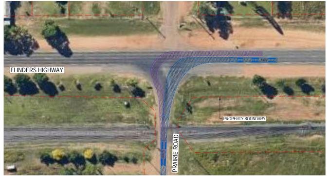
26m B-DOUBLE ENTERING EAST/ 8.8m SERVICE VEHICLE EXITING EAST SCALE 1:500 (m)
