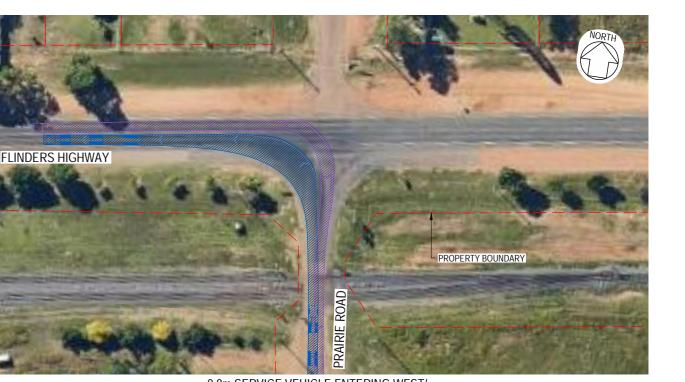
8.8m SERVICE VEHICLE ENTERING WEST/ 26m B-DOUBLE EXITING WEST SCALE 1:500 (m)
