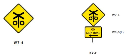
Figure 23: Railway crossing ahead active control signs
