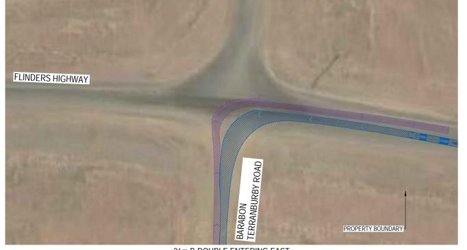
26m B-DOUBLE ENTERING EAST 8.8m SERVICE VEHICLE EXITING EAST SCALE 1:500 (m)
