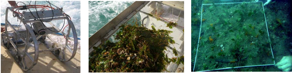
Figure 2. Sampling sites were assessed by deep water sled tows with CCTV mounted camera system and free-divers to measure seagrass biomass and species composition.
