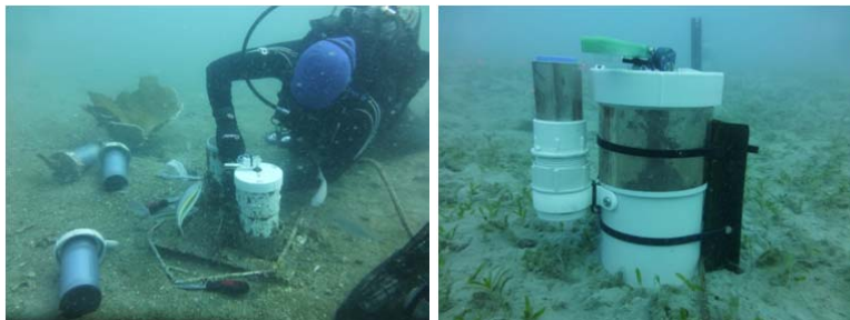
Figure 3. Diver deploying PAR loggers and associated wiper units
