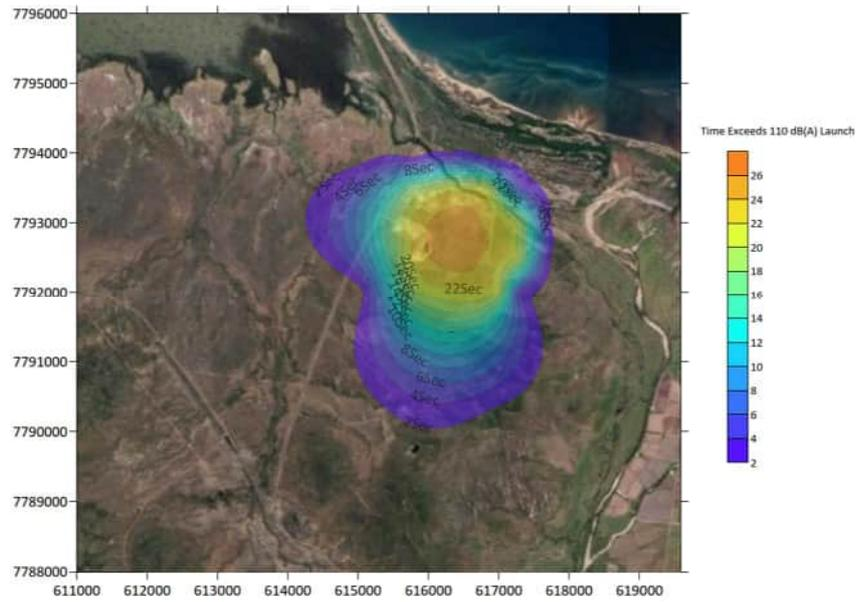
Figure 7 Time exceeding 110 db(A) during launch
