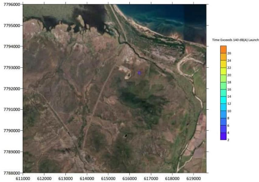
Figure 9 Time exceeding 140 db(A) during launch
