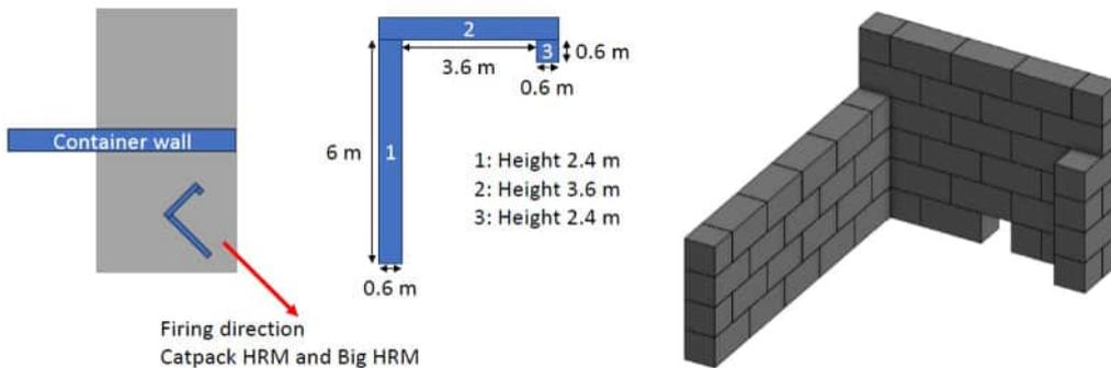
Figure 3 Link Block Walls Test Stand 1A
