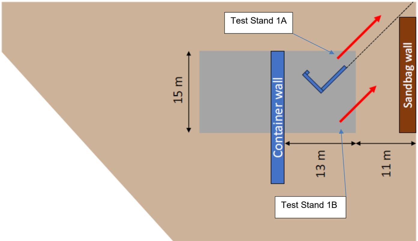
Figure 2: Test Pad 1 Showing Engine Stands, Container wall and 20m long Sandbag wall.
