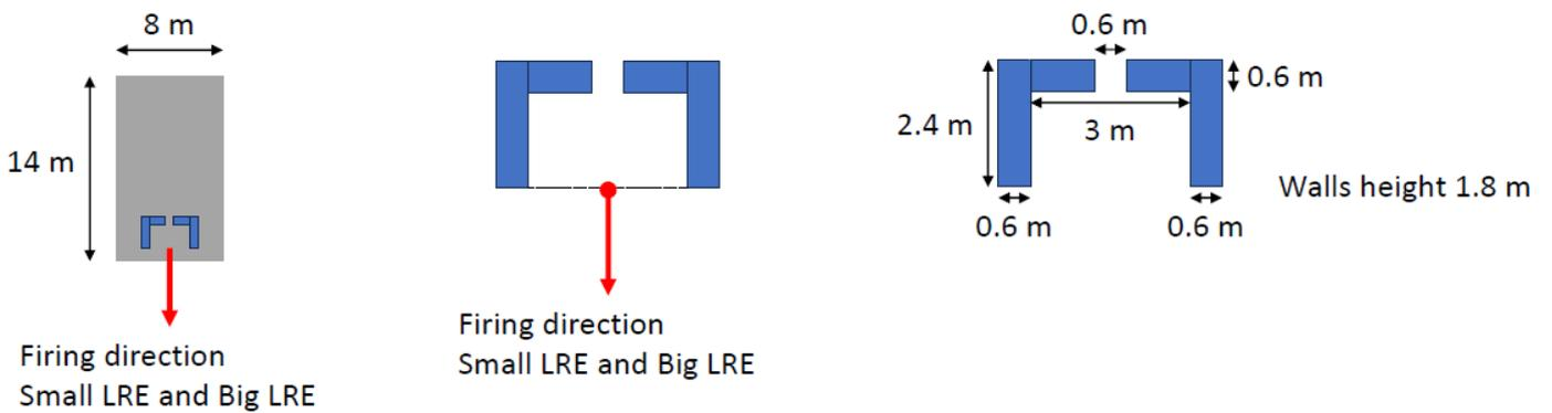
Figure 5: Test Pad 2 Link Block Walls Description
