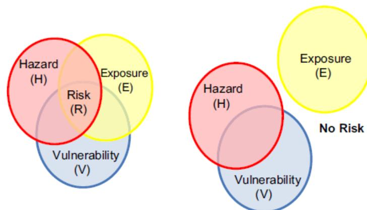
Figure 6 Representation of how Exposure Removal through Implementation of Exclusion Zone Lowers Risks
