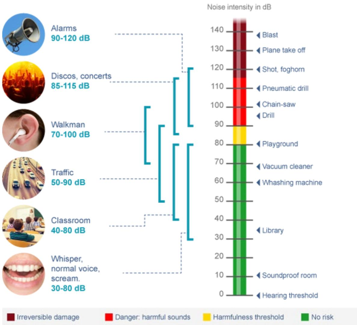
Figure 6: Examples of Noise Sources and Sound Pressure Levels(Source Cochlea.org)
