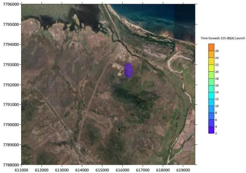
Figure 8 Time exceeding 125 db(A) during launch
