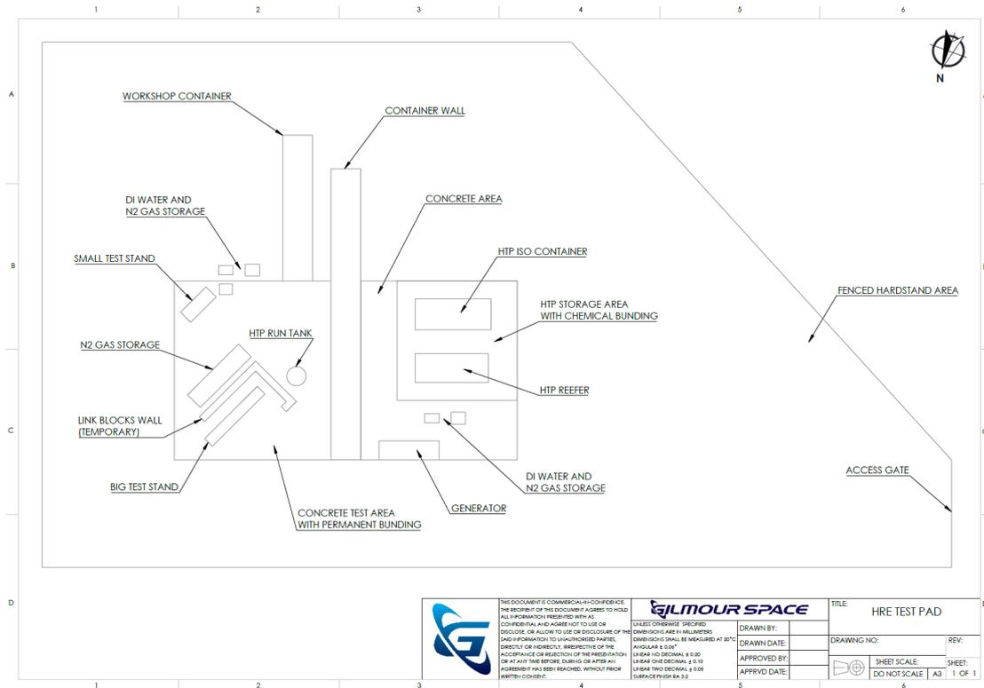
Figure 8 - HRE Test Pad Typical Layout
