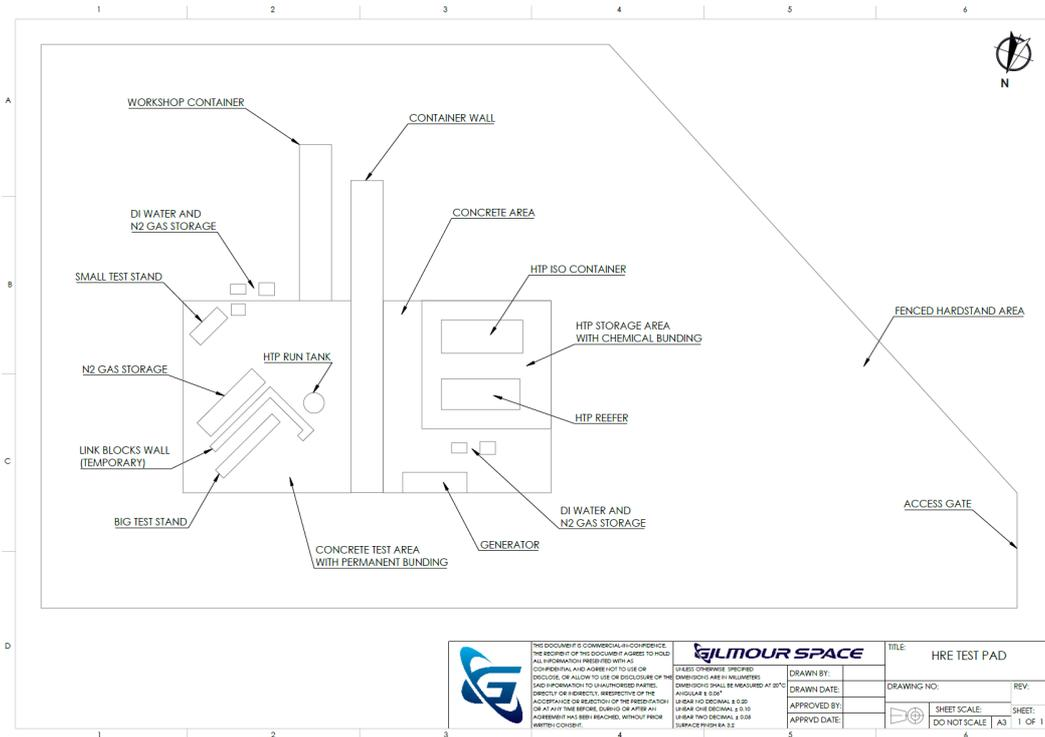
Figure 4 - HRE Test Pad Typical Layout
