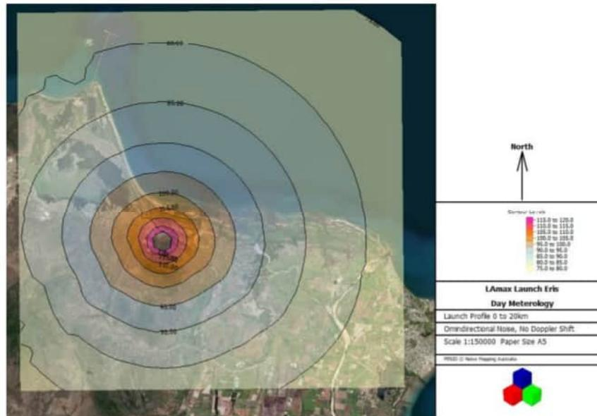
Figure 10 Peak sound exposure  $L_{Amax}$
