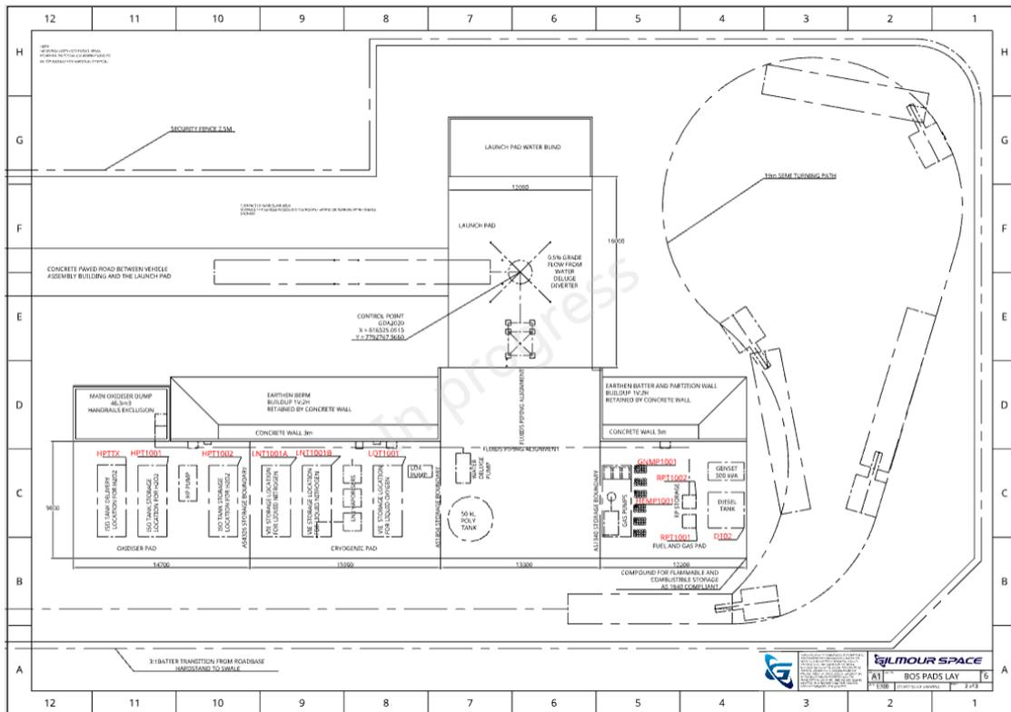
Figure 3 - Hazardous and Dangerous Goods Storage Areas Layout for Launch Pad and Storage Pads
