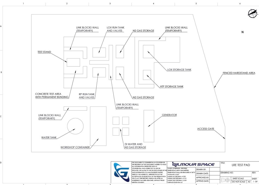
Figure 5 - LRE Test Pad Typical Layout
