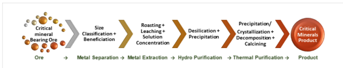
Figure 3 Draft Mineral Recovery Process
