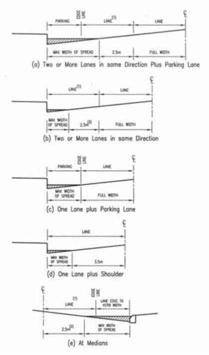
Figure 10 Allowable flow widths - 10% AEP flood (TMR Road Drainage Manual)
