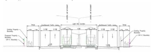
Figure 15 Typical LRT cross-section at stations
