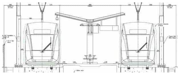
Figure 29 Typical island platform cross section
