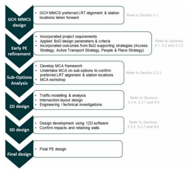
Figure 16 LRT Option - PE design development process
