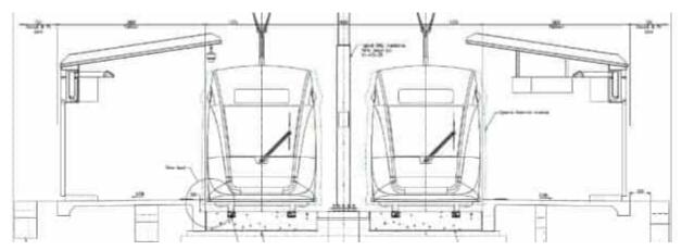
Figure 28 Typical side platform cross section
