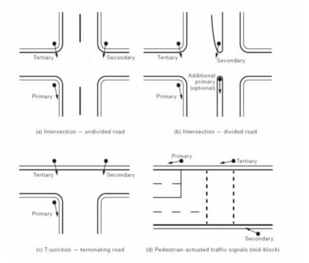
Figure 11 Minimum traffic signal layout
