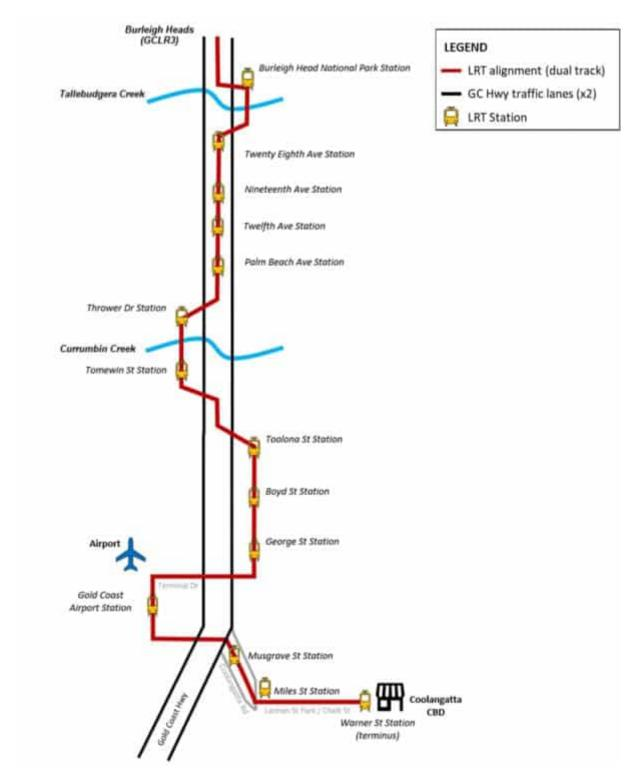
Figure 12 Schematic of the preferred GCH MMCS LRT alignment and station locations
