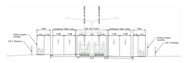
Figure 14 Typical LRT cross-section with centre running
