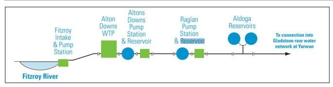
Figure 2.1 Schematic of key project infrastructure
