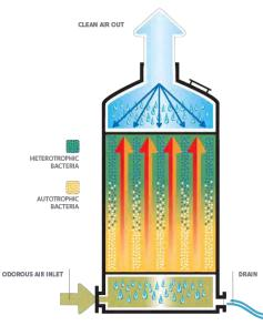
Figure 1 Schematic EcoFilter
