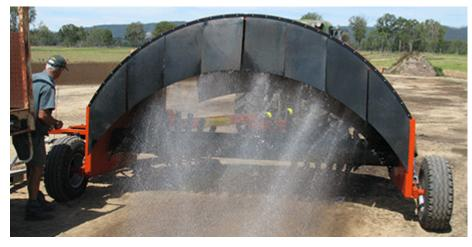
Figure 56. Compost is wetted while being turned to reduce dust
