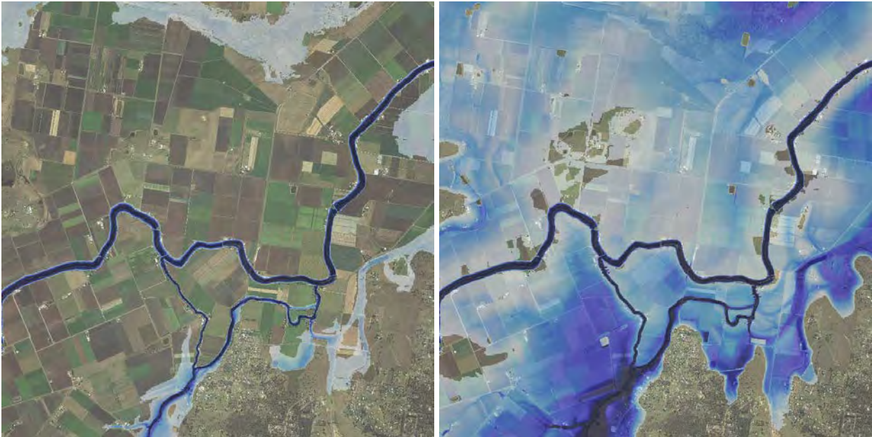
Figure 5.1 Flow patterns around the Glenore Grove gauge site for low and high flows
