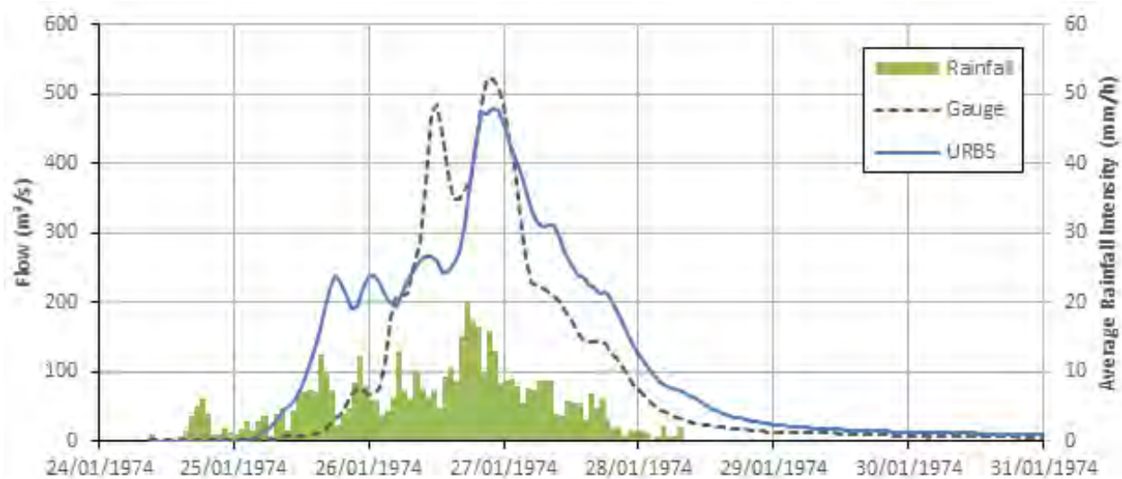
Figure 7.33 Comparison of URBS and stream gauge hydrographs at Adam's Bridge for the 1974 event
