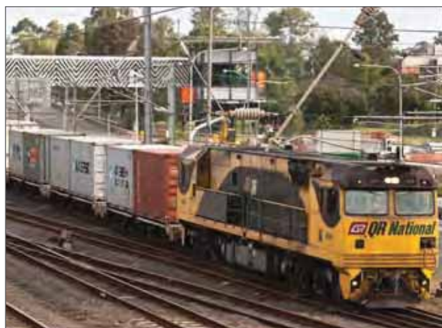
Freight rail, dual gauge track, Yeerongpilly
