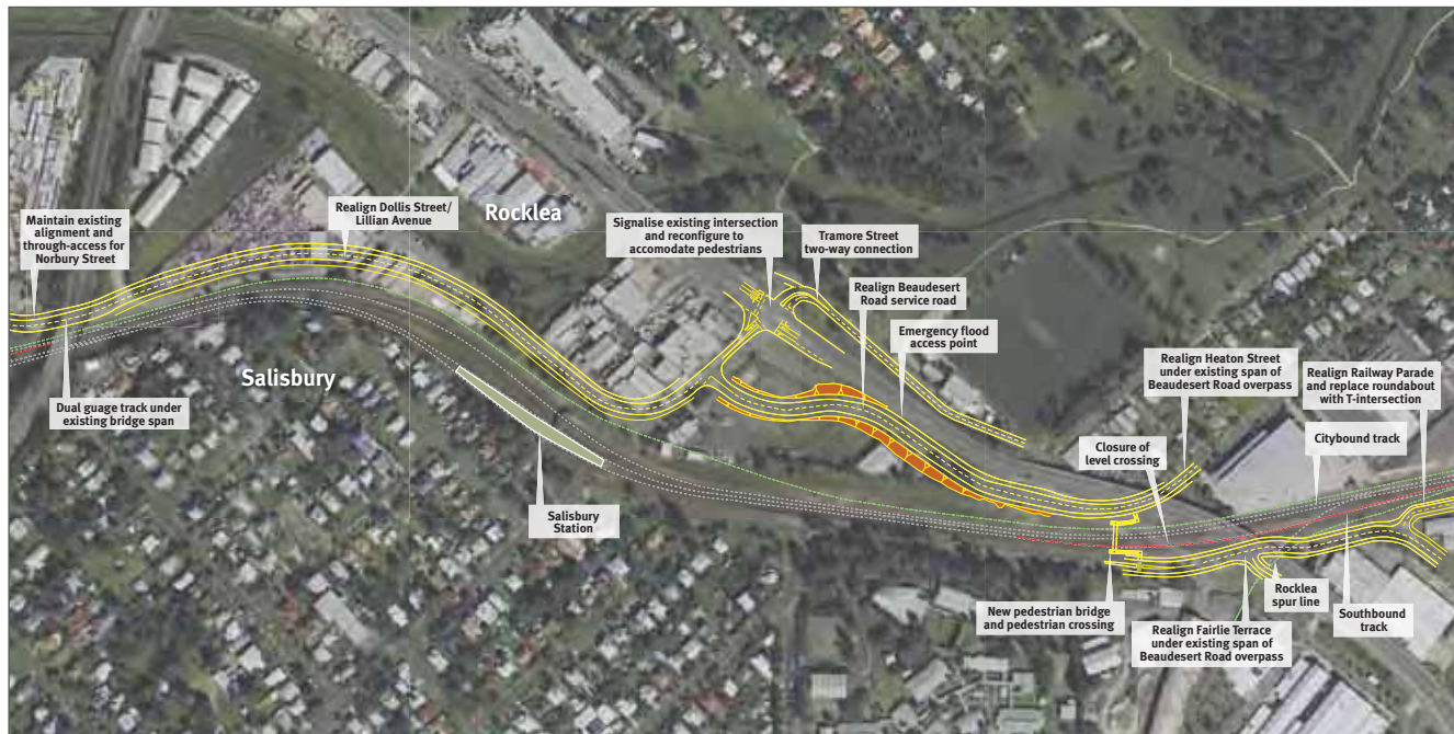
Figure 2-4 Southern road works
