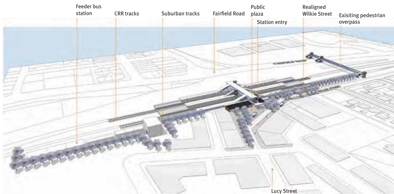
Figure 2-13 Yeerongpilly Station – indicative view looking west
