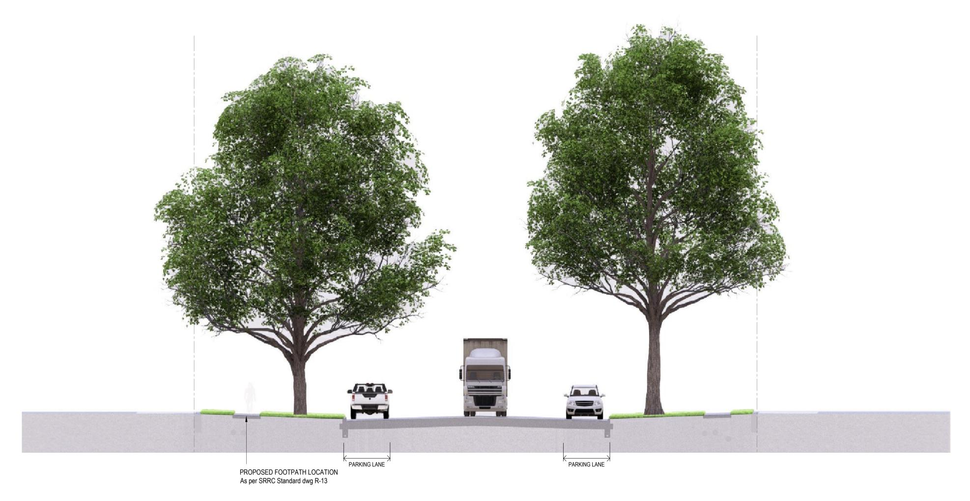
2 TYPICAL ROAD CROSS SECTION - NEW ROAD 2 SCALE 1:100 @ A1
