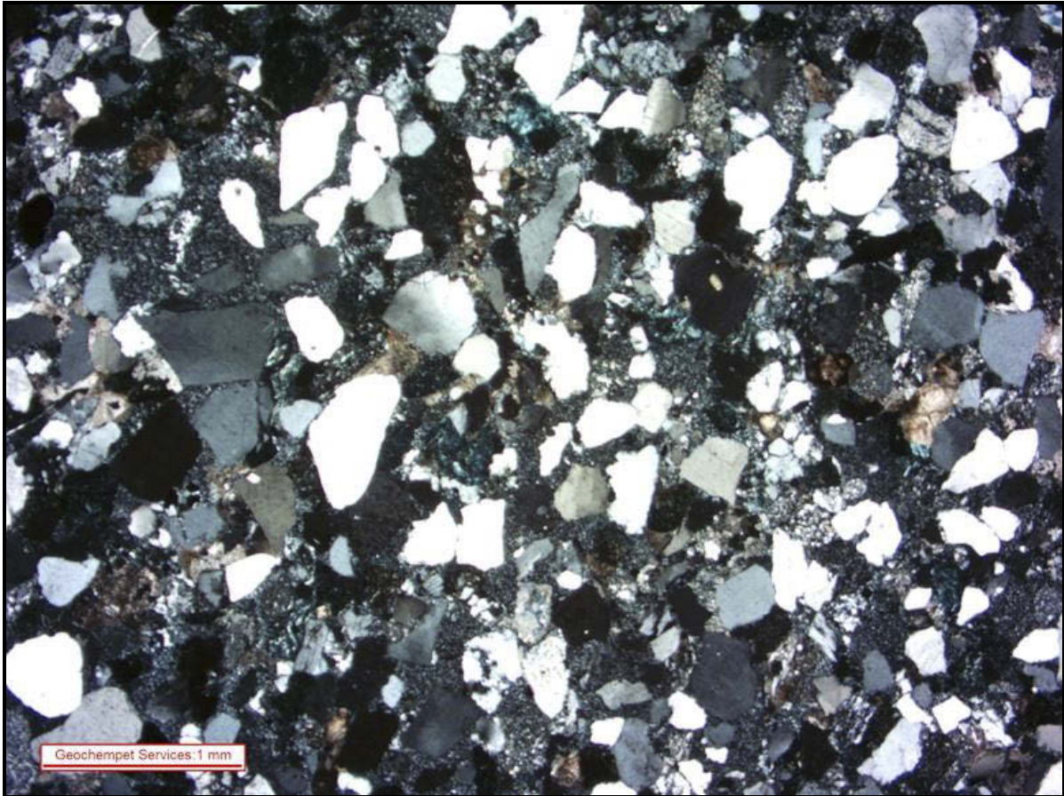
Plate 2: Micrograph taken at low magnification in transmitted cross polarised light of part of the sandstone. Image shows quartz, feldspar and lithic grains along with part of the matrix being slightly carbonated.
