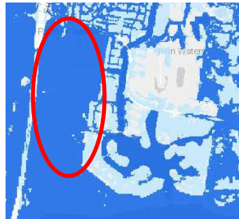
Figure 1 SCC flood hazard mapping of the site and adjacent vulnerable area: dark blue shows flood modelling under current climate; Light blue extends the area under future climate http://maps.sunshinecoast.qld.gov.au/maplet/index.html?config=config/mymaps/myplace/FloodHazardArea.xml
