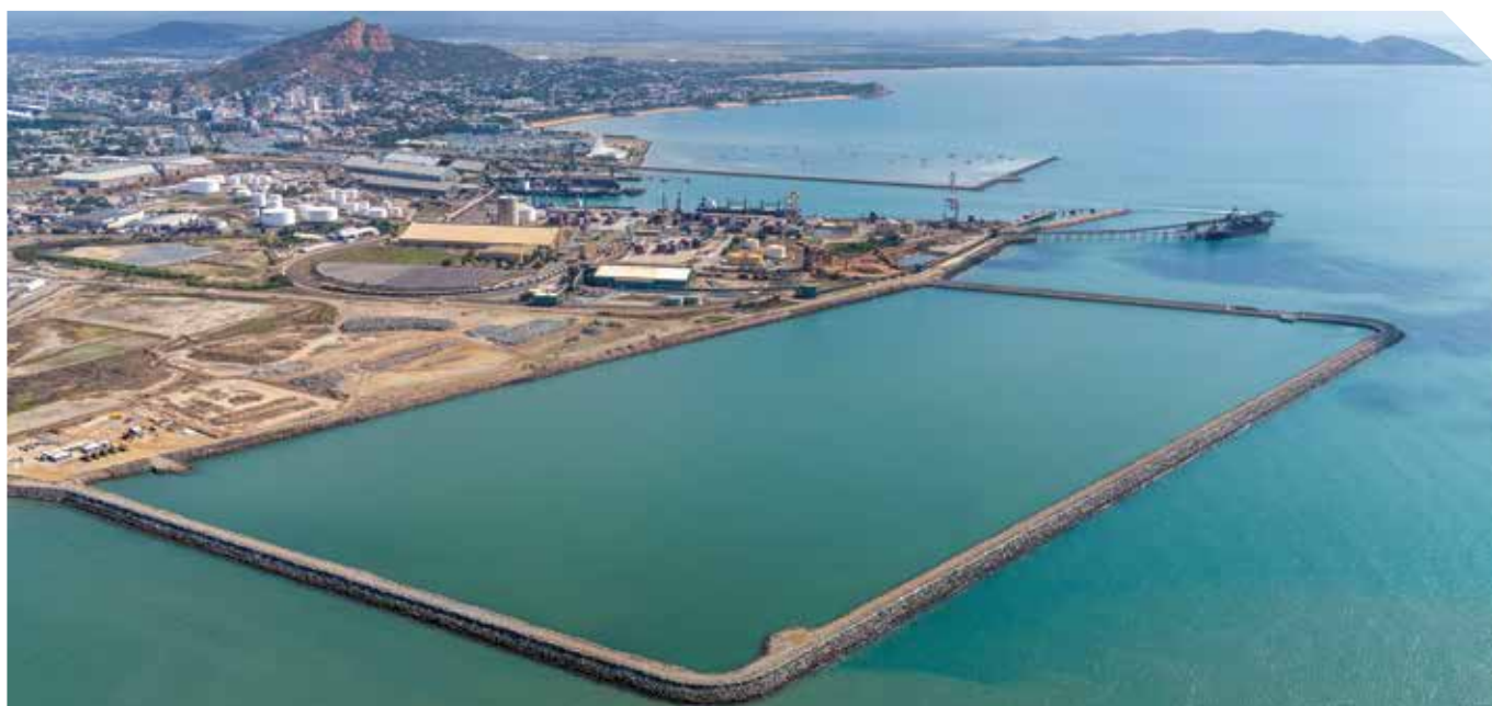
The $232 million Channel Upgrade project has marked a major milestone with the completion of the 2.2km rock wall, which forms the boundary of a 62ha reclamation area.
