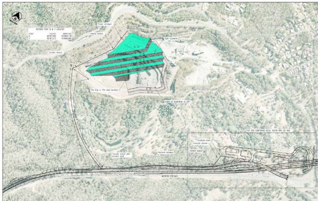
Figure 4.2 Changed project—spoil conveyor route and stockpile design
