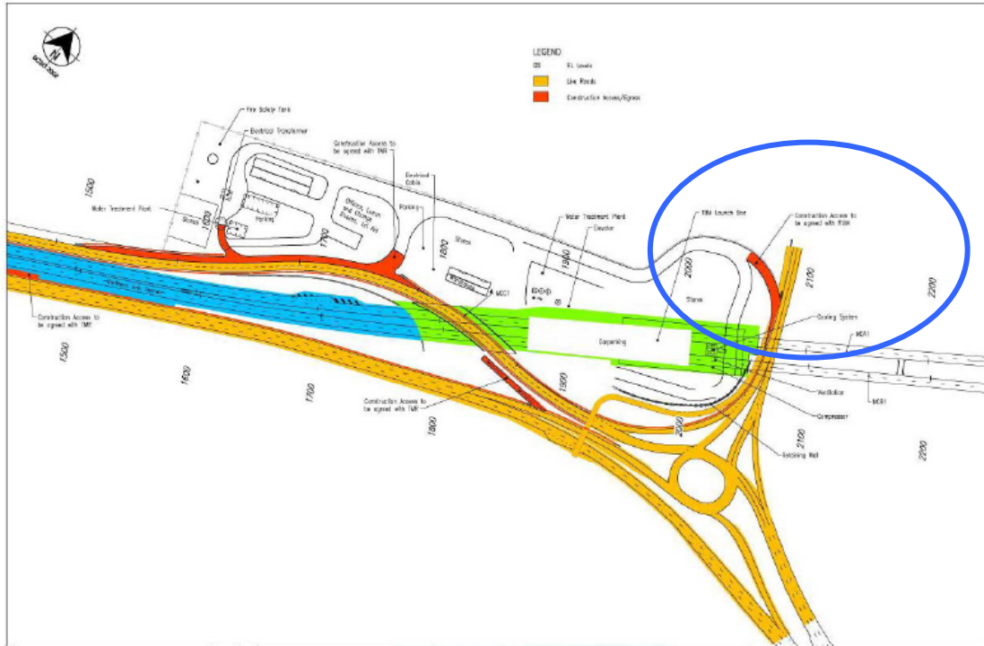
Figure 4.1 Western worksite (light vehicle access circled)
