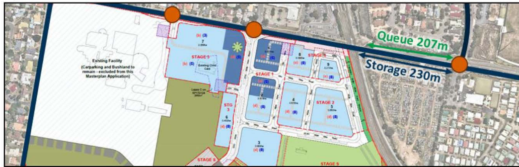
Figure 4-9 Intersection Separation to Train Crossing
