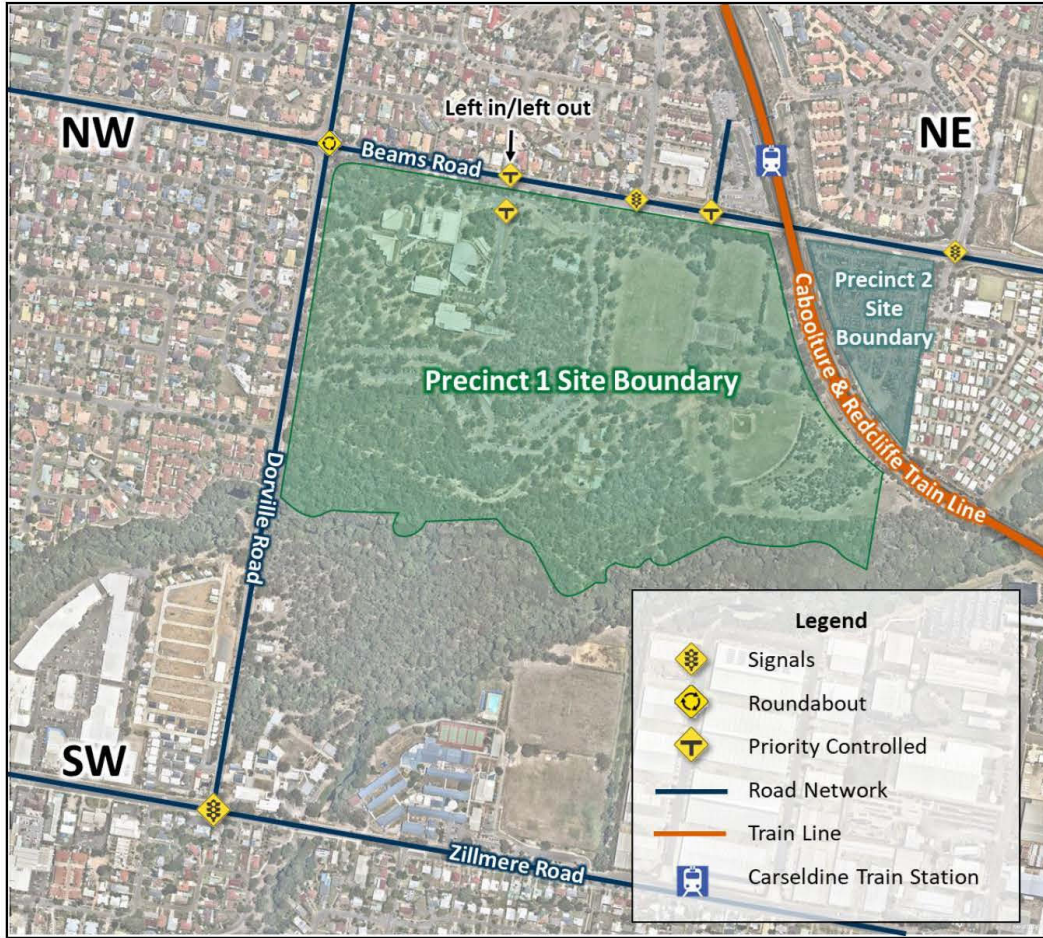
Figure 3-6 Intersection Control Types
