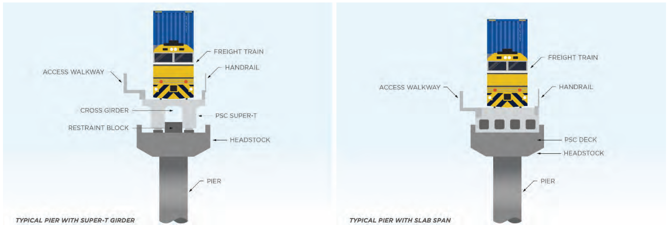
FIGURE 8: TYPICAL PIER WITH PRE-STRESSED CONCRETE SUPER-T GIRDER (LEFT); TYPICAL PIER WITH PRE-STRESSED CONCRETE SLAB SPAN (RIGHT)
