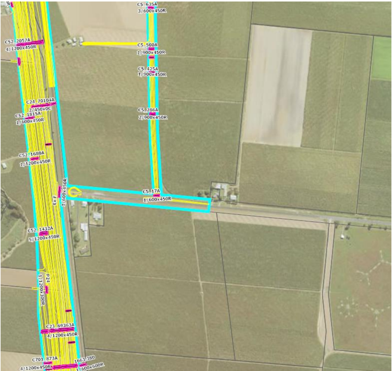
Figure 2 Cross Drainage structures E2G
