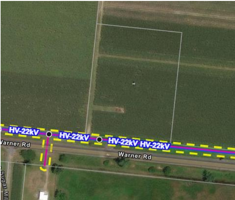
Figure 10 Existing High Voltage and low Voltage Electricity Supply Warner Road, Source: Ergon look up and Live
