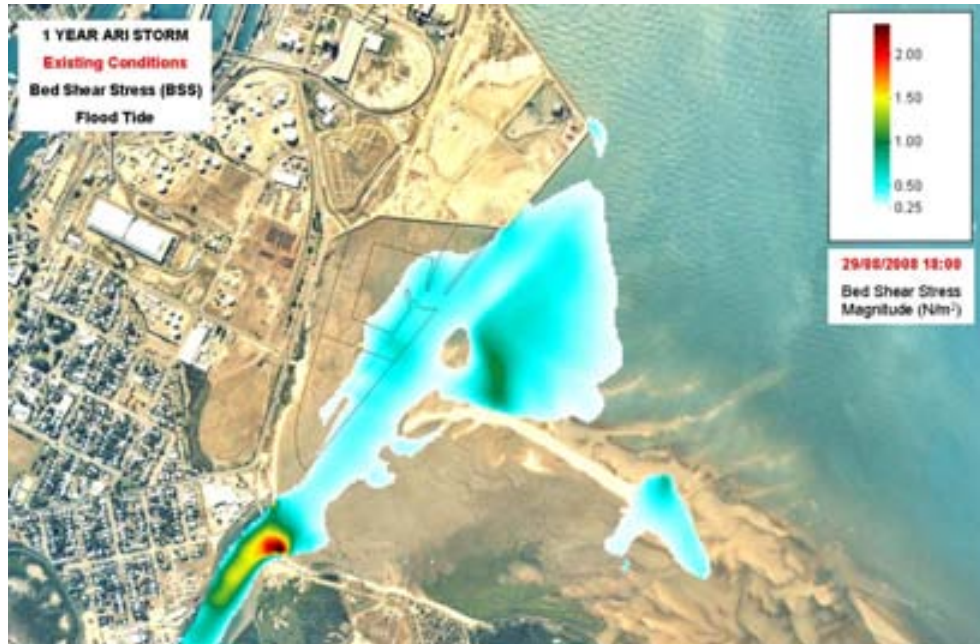
Figure 3-38 Existing bed shear stresses for storm wave (1 year ARI) conditions.
