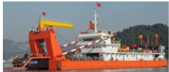
Medium sized cutter suction dredge
