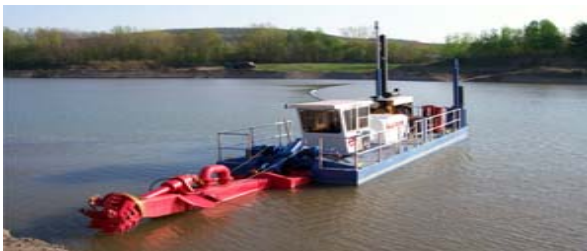
Small sized cutter suction dredge
