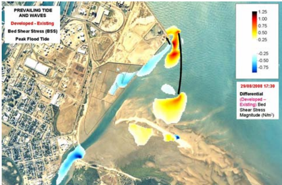
Figure 3-36 Differential of bed shear stresses during flood phase of spring tide (prevailing scenario) for developed conditions.
