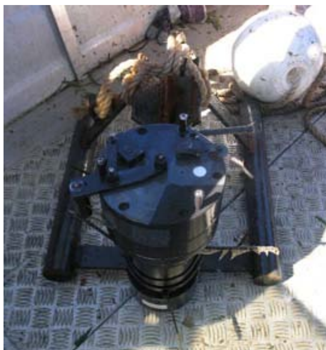
Figure 3-51 Sedentary Water Quality Logger Prior to Deployment
