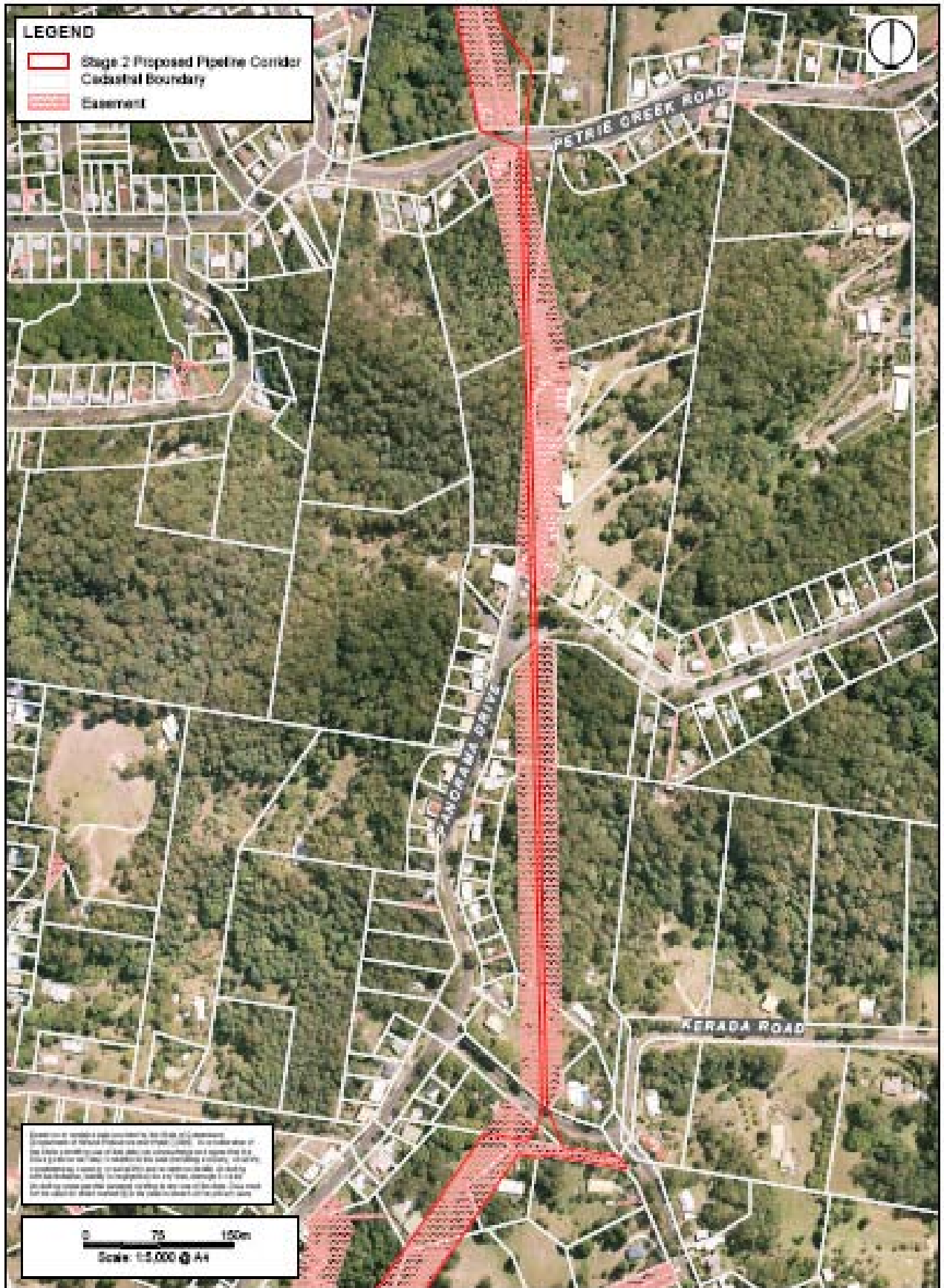
Figure 11 Pringle Hill tunnel alignment
