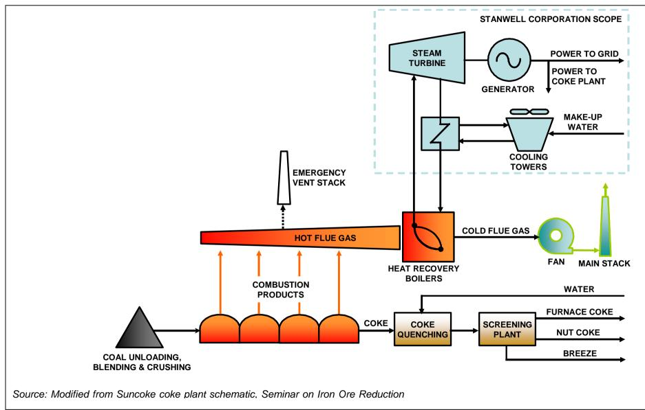
Figure 4: Coke Power Project Simplified Process
