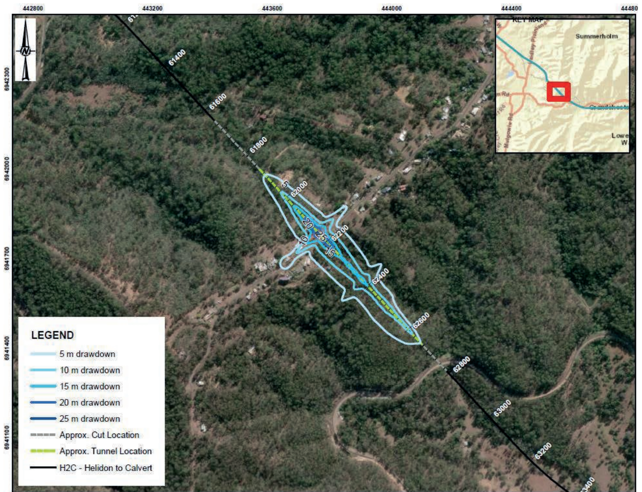
Figure 20: Estimated drawdown of groundwater table between Kilometrage 61.600 and 62.800 km due to drainage of the Little Liverpool Tunnel (Scenario 3).
