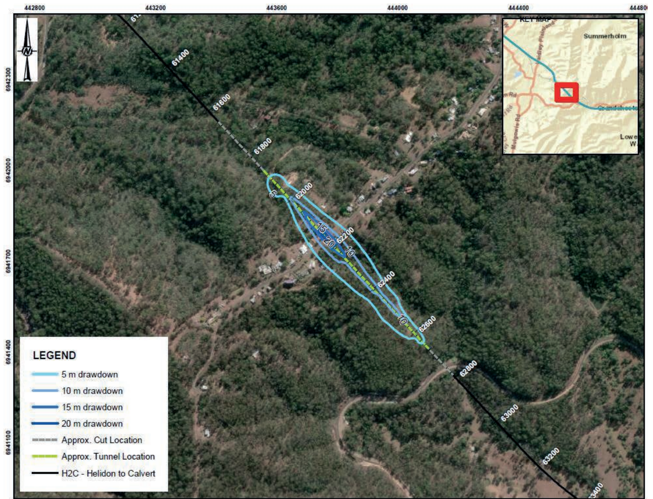
Figure 18: Estimated drawdown of groundwater table between Kilometrage 61.600 and 62.800 km due drainage of the Little Liverpool Tunnel (Scenario 1).
