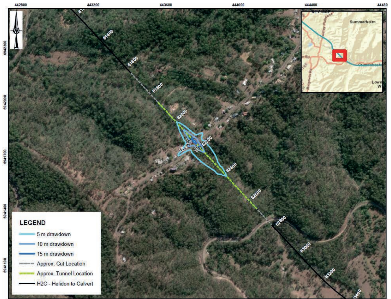
Figure 19: Estimated drawdown of groundwater table between Kilometrage 61.600 and 62.800 km due to drainage of the Little Liverpool Tunnel (Scenario 2).
