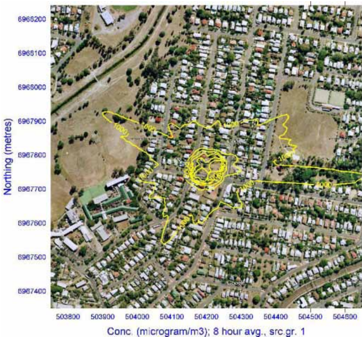
Figure 5: Predicted Cumulative Ground Level CO Concentrations (8-hour Average) (µg/m 3 ), Air Quality Goal – 11,000 µg/m 3
