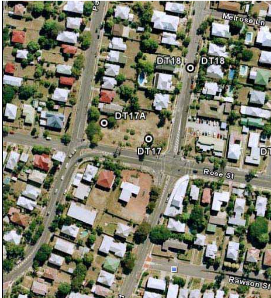
Figure 5 – Groundwater Borehole Locations
