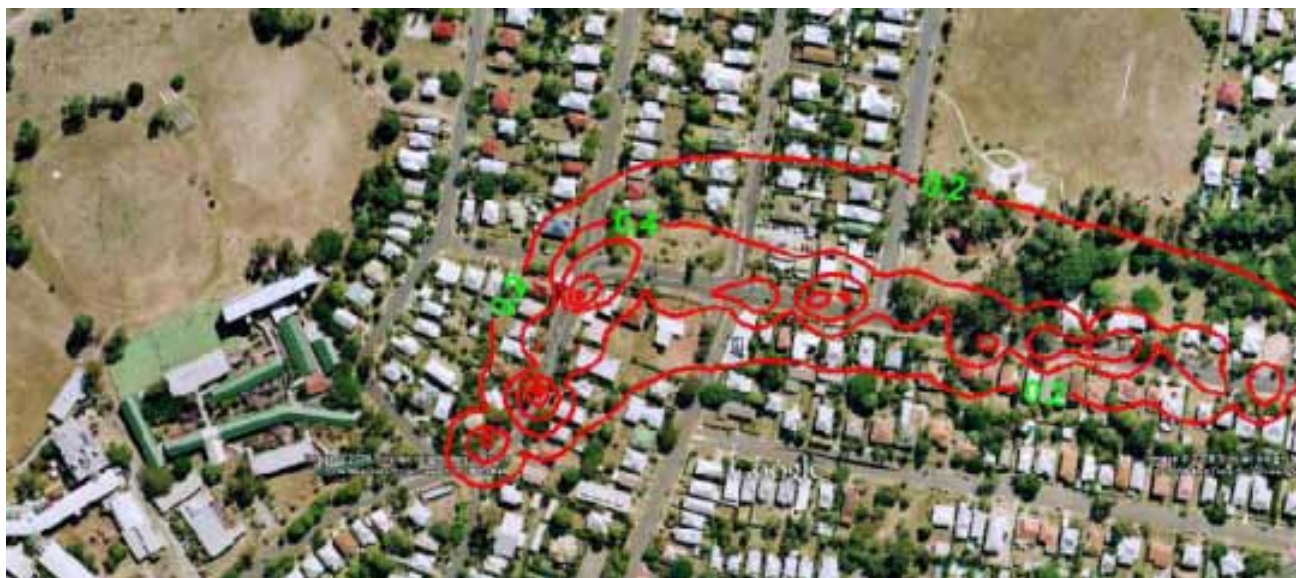
Figure 15a: Existing Traffic - Predicted Ground Level Benzene Concentrations (Annual Average) ( \mu\text{g}/\text{m}^3 )
