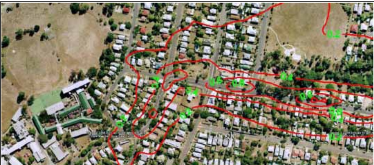
Figure 13b: Contribution from Haul Vehicles - Predicted Ground Level PM 10 Concentrations (24-hour Average) ( \mu\text{g}/\text{m}^3 )
