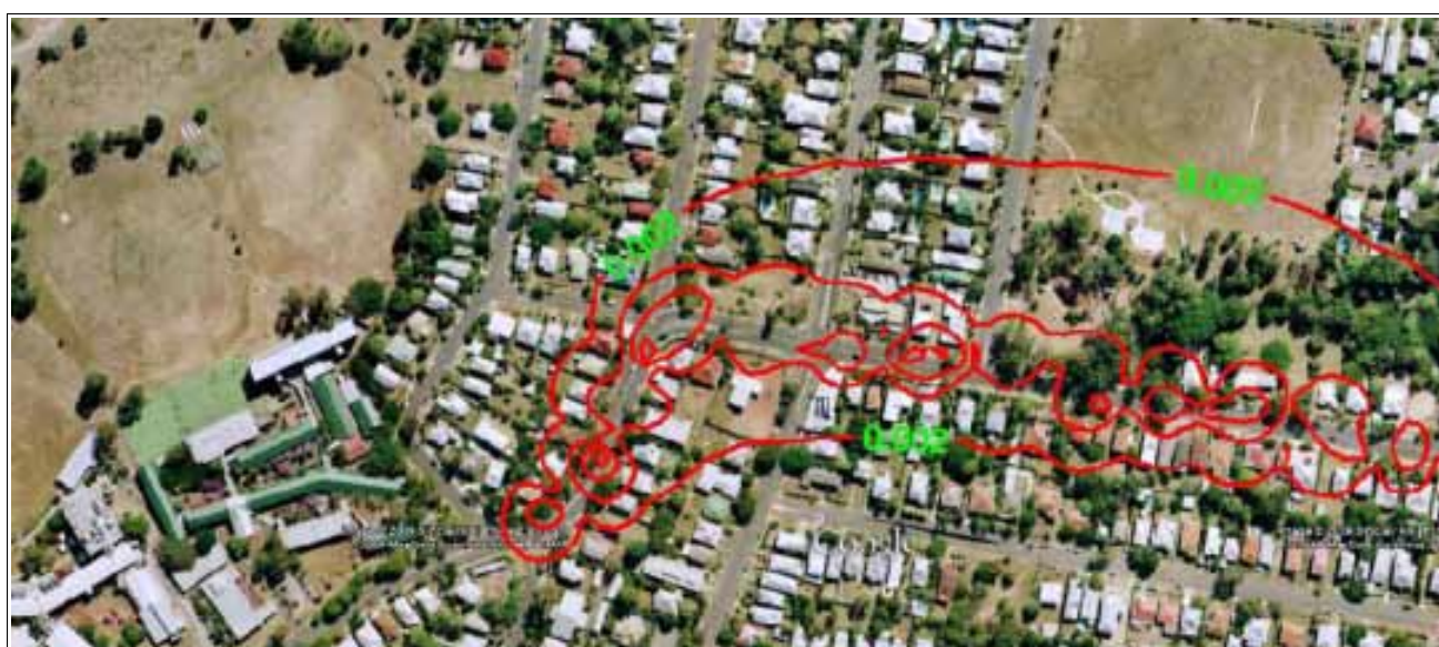
Figure 15b: Contribution from Haul Vehicles - Predicted Cumulative Ground Level Benzene Concentrations (Annual Average) ( \mu\text{g}/\text{m}^3 )
