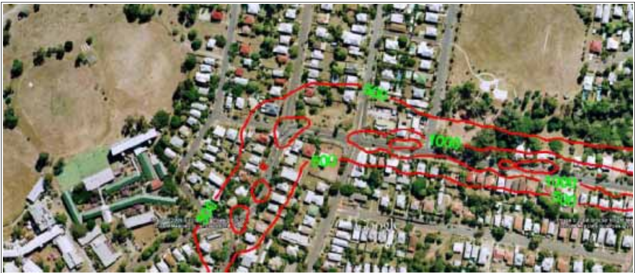
Figure 16a: Existing Traffic - Predicted Cumulative Ground Level CO Concentrations (8-hour Average) ( \mu\text{g}/\text{m}^3 )
