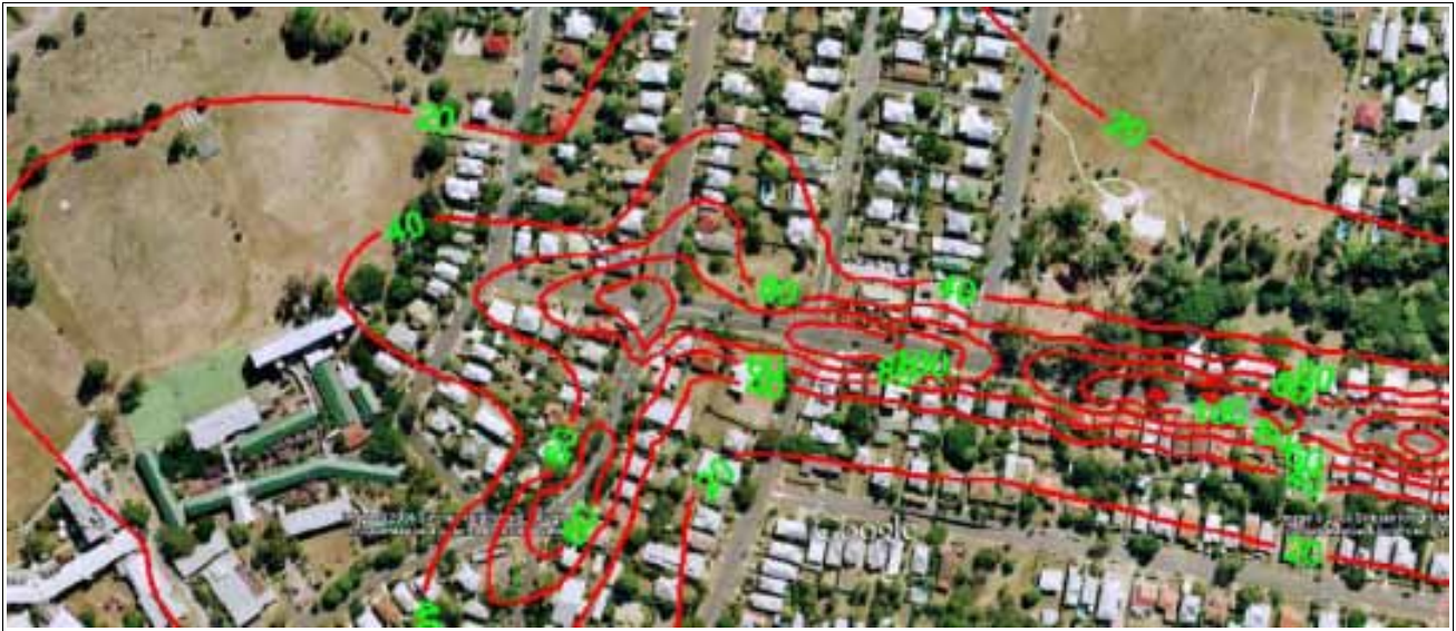
Figure 14a: Existing Traffic - Predicted Ground Level NO 2 Concentrations (1-hour Average) ( \mu\text{g}/\text{m}^3 )
