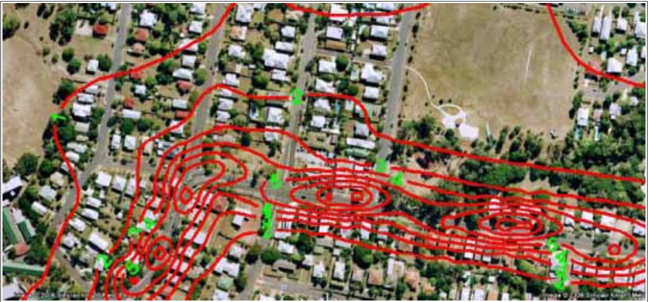
Figure 13a: Existing Traffic - Predicted Ground Level PM 10 Concentrations (24-hour Average) ( \mu\text{g}/\text{m}^3 )
