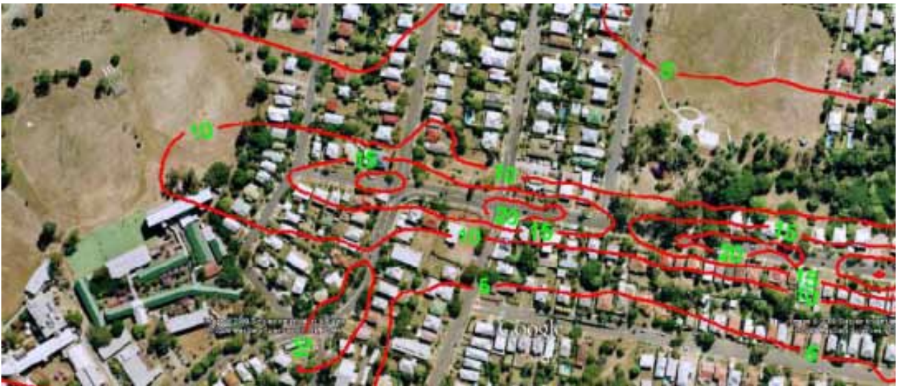
Figure 14b: Contribution from Haul Vehicles - Predicted Ground Level NO 2 Concentrations (1-hour Average) ( \mu\text{g}/\text{m}^3 )
