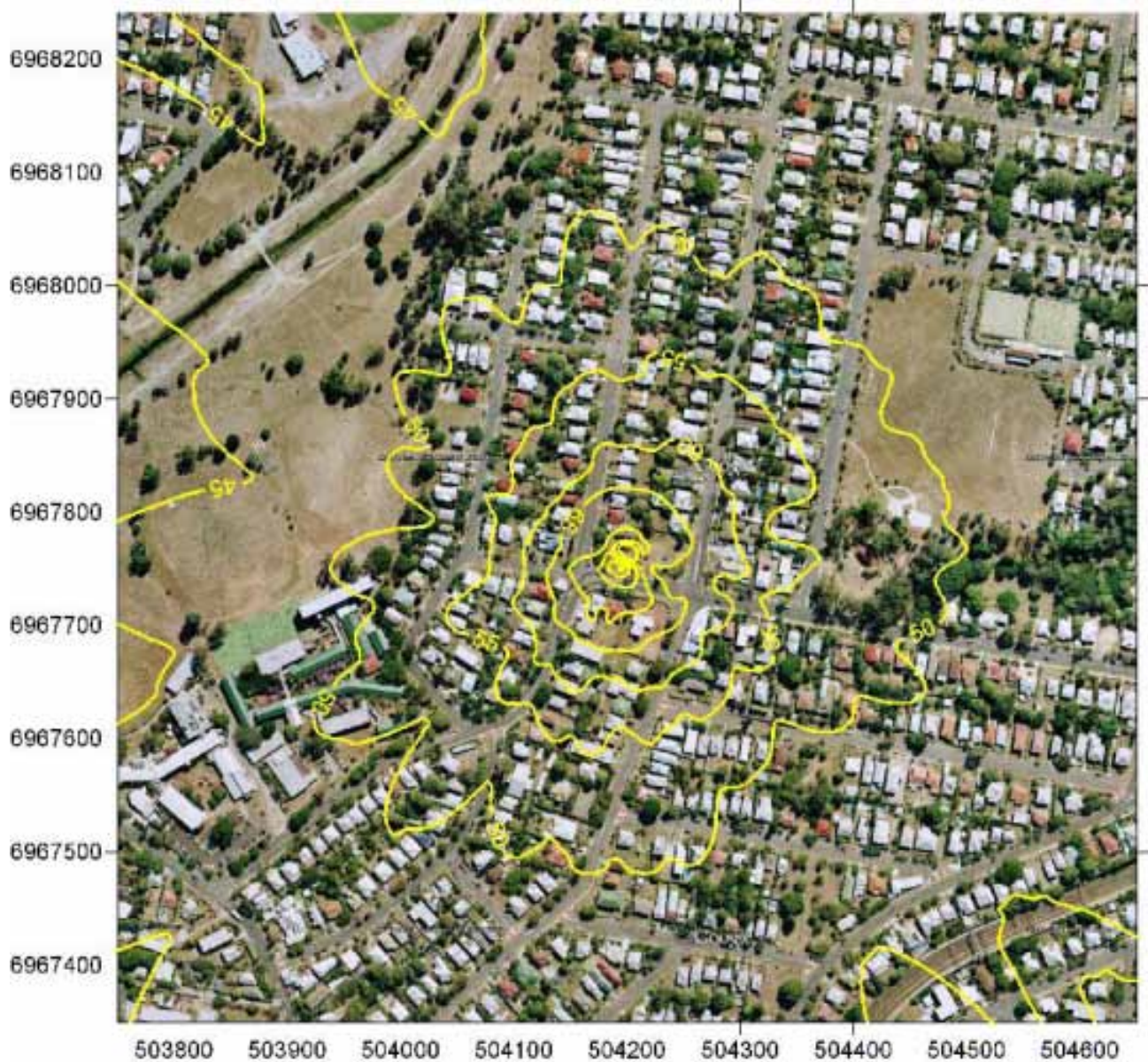
Figure 2: Predicted Cumulative Ground Level NO 2 Concentrations (1-hour Average) ( \mu\text{g}/\text{m}^3 ), Air Quality Goal – 246 \mu\text{g}/\text{m}^3
