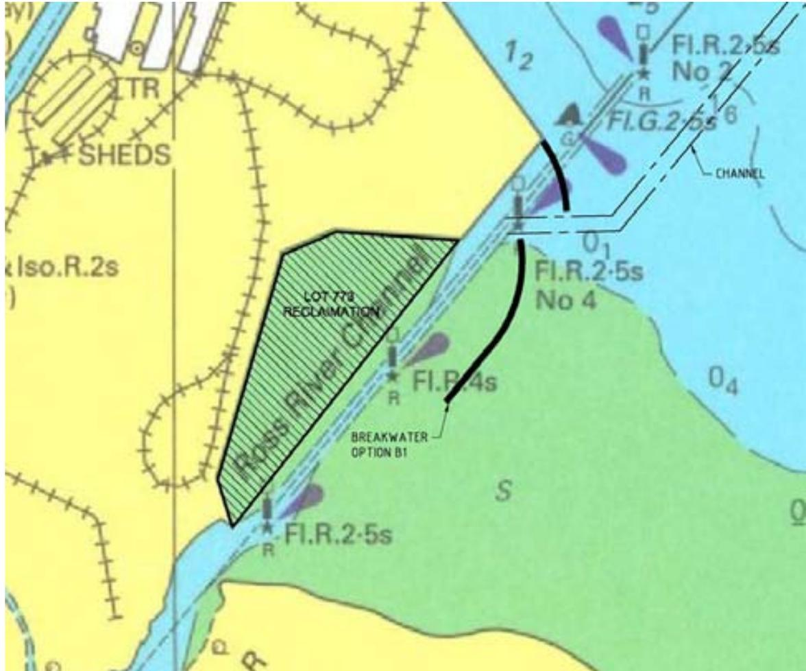
**Option B** is characterised by breakwater protection extending alongside the Marine Precinct reclamation lot 773 with an additional breakwater extension adjacent the end of the Eastern Reclaim Area. The option was selected as a refinement of TOR option Min and features a split breakwater providing additional protection from the predominant wave direction and reducing the impact on the mudflats to the east of Ross River.
