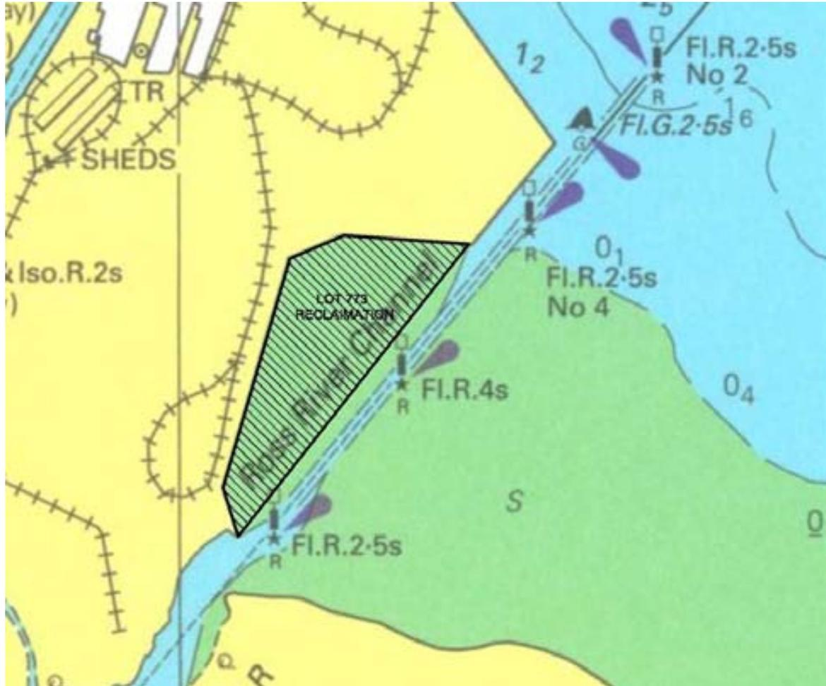
Option **No Breakwater – continuous quayline** is an option which provides a maximum area of reclaimed land within the Precinct area. This option requires the external quayline to be utilised as the “working” face for marine industries within the precinct. The precinct reclamation configuration provided by this configuration has been adopted as the base case for the reclamation configuration in all of the breakwater options assessed.
