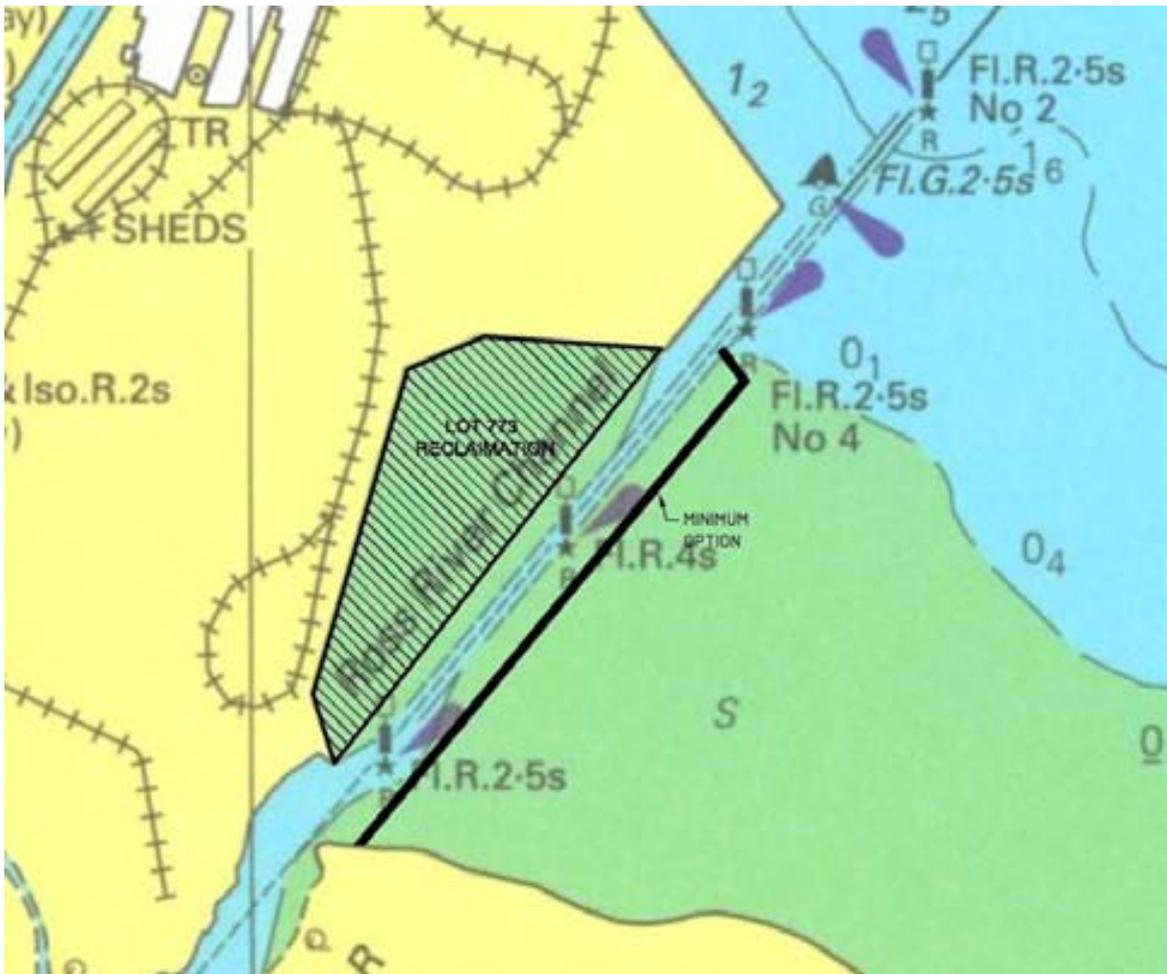
Option **Min** is characterised by breakwater protection extending alongside the Marine Precinct reclamation with a partial return just beyond the seaward extent of lot 773. The option isolates the Ross River navigation channel from the mud flats to the east and provides an obstacle to littoral transport from the beaches to the East of the development.
