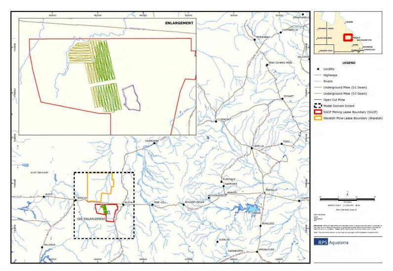
Figure 5.5 South Galilee Coal Project groundwater model boundaries
