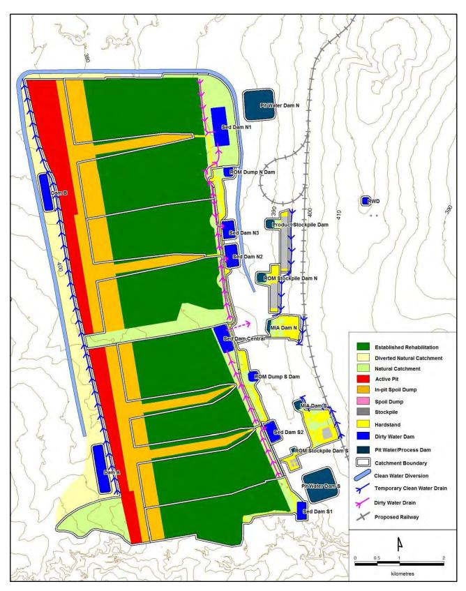
Figure 5.7 Mine arrangement and water management system
