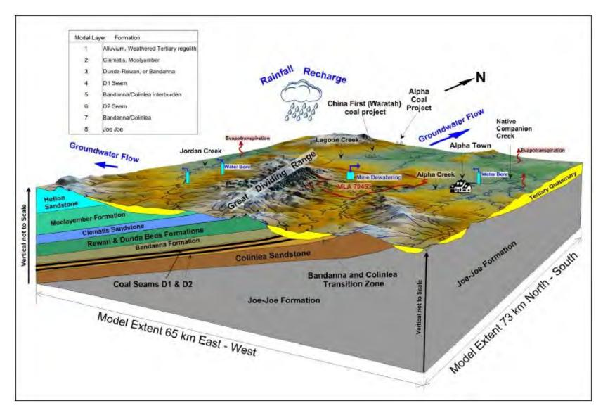
Figure 5.4 Conceptual groundwater model
