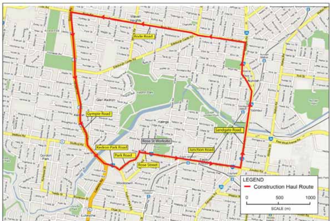
Figure 8-1: Construction Haul Route for Rose Street Worksite
