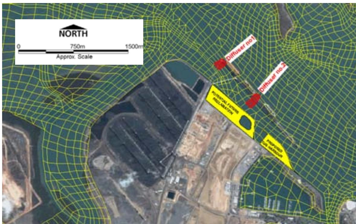
**Figure 7-12 Model Elements Selected to Represent Diffuser Lines. Stage 1 Employed Diffuser 1 Only, and Stage 2 Employed all Diffusers**
