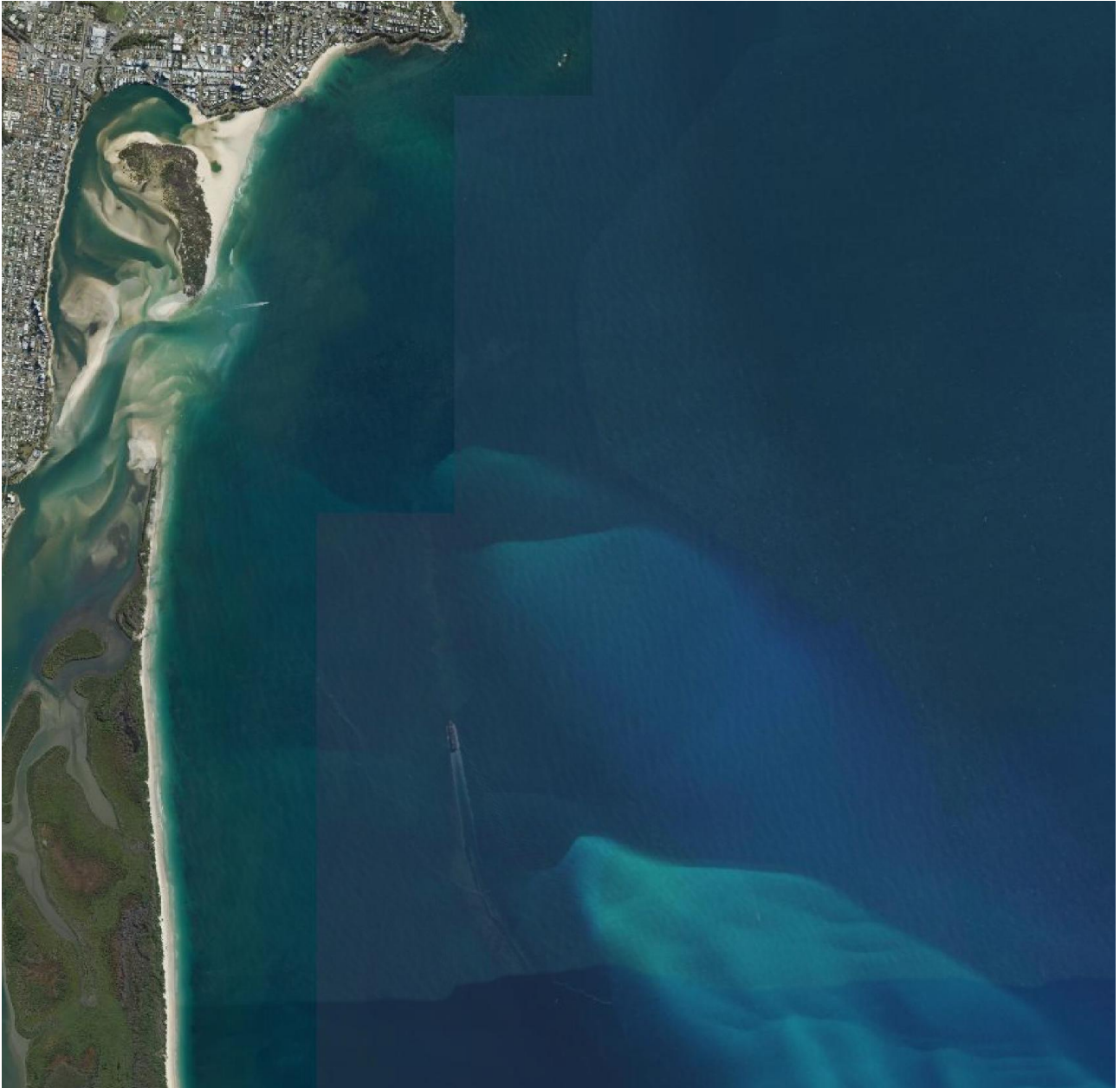
Figure 46: Northward transport pattern suggested for tip of North Banks and Hamilton Patches (Qld Globe)
