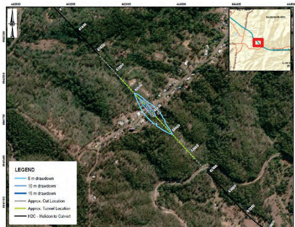
FIGURE 14.9: BASE CASE: ESTIMATED LONG-TERM DRAWDOWN AT LITTLE LIVERPOOL RANGE TUNNEL
