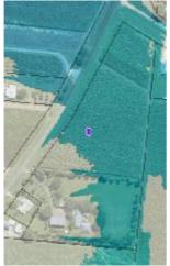
Figure 1 shows the extent of inundation during a 1% AEP flood event
