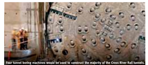
Four tunnel boring machines would be used to construct the majority of the Cross River Rail tunnels.
