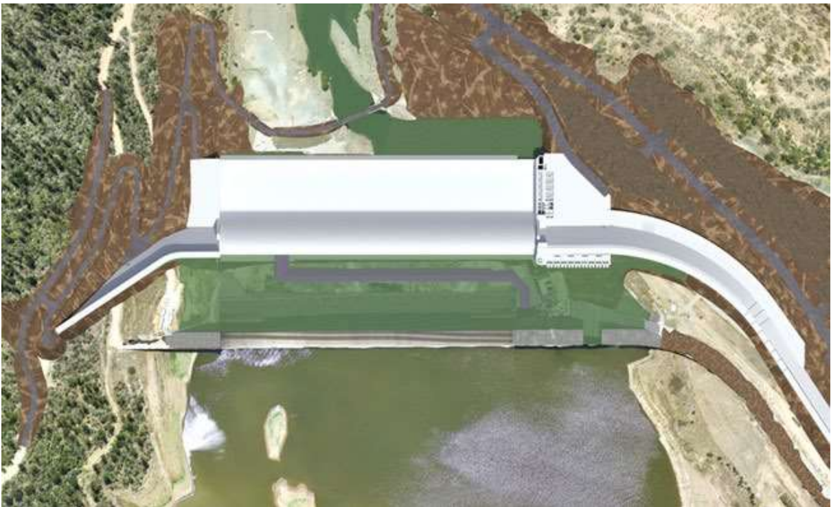
Figure 6. Conceptual view of the replacement dam wall downstream of existing Dam structure (view is shown looking downstream)
