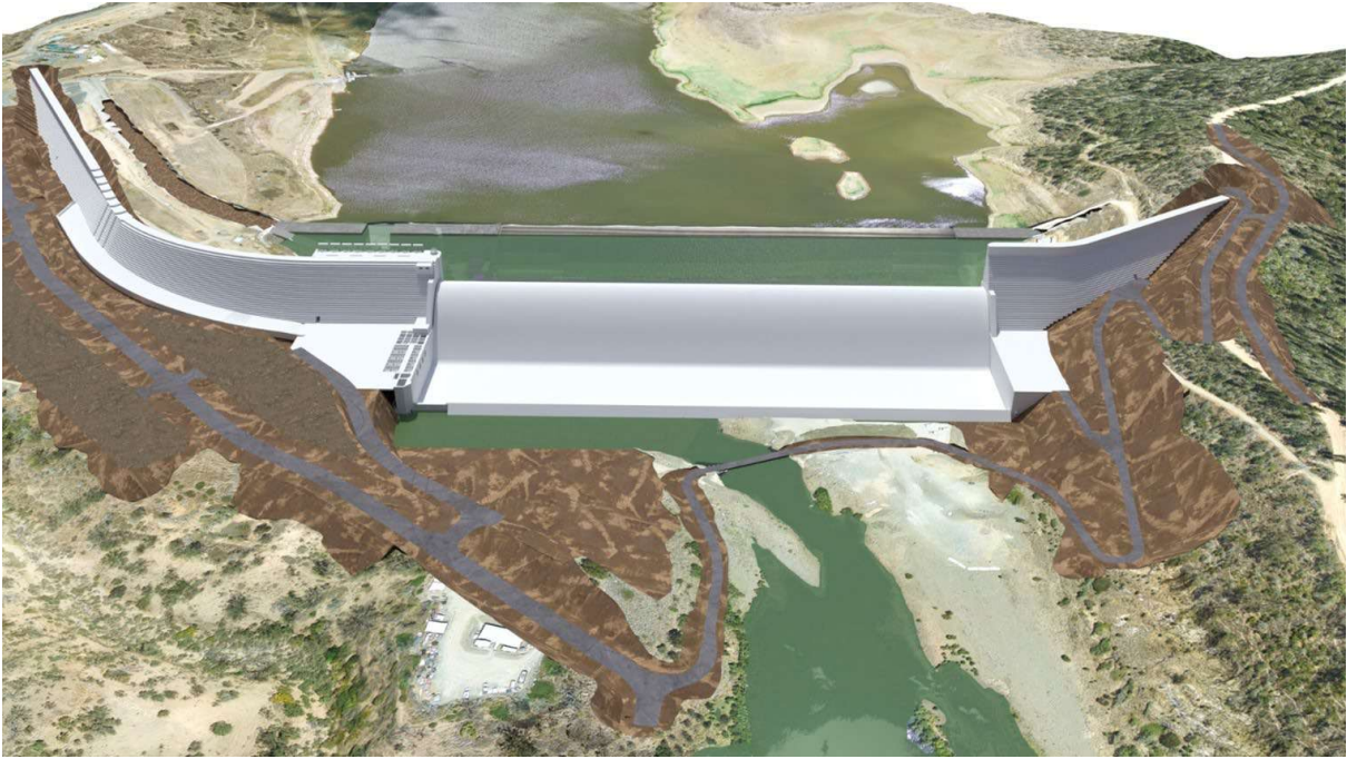
Figure 5. Conceptual view of the replacement dam wall downstream of existing Dam structure (view is shown looking upstream)
