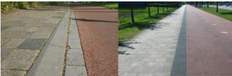
Figure 8-21 Diagonal Edge and No Edge Treatment for Pedestrian Path/Cycle Track Transition
