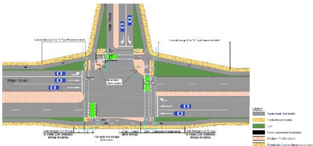
Figure 8-13 Typical Layout at Signalised T-Intersection
