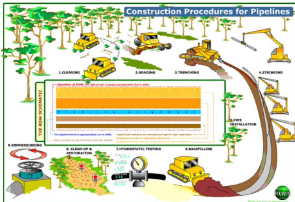
Figure 4-4: Construction Procedures for Pipelines (Source: RLMS)
