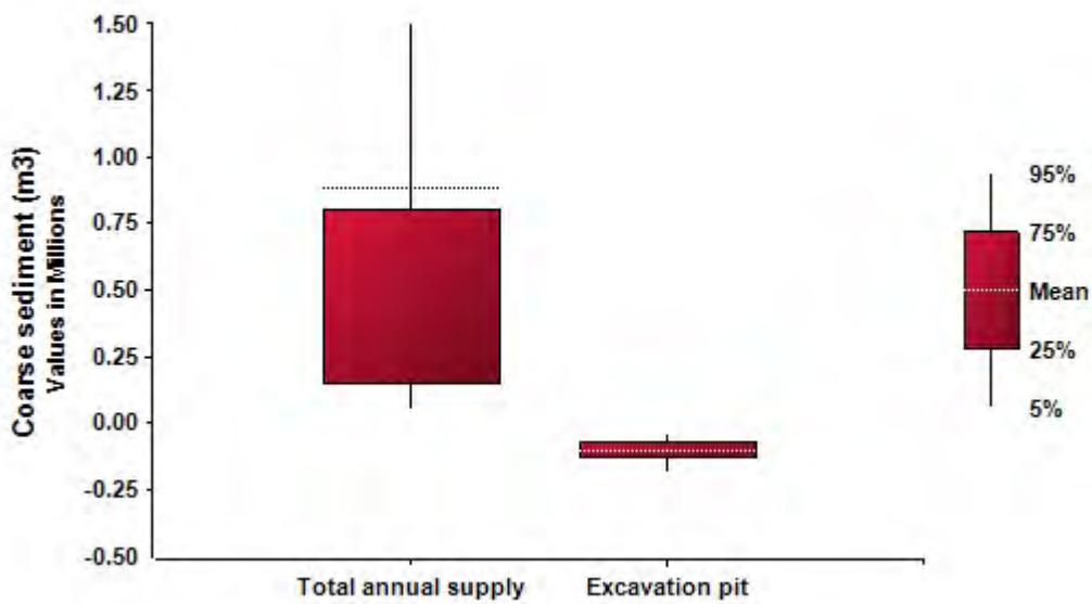
Figure 3-13 Comparison between total coarse material supply (TCL) and proposed extraction in Denison Creek
