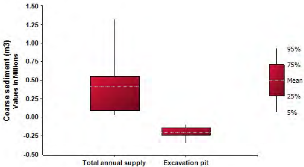
Figure 3-21 Comparison between total annual supply (TCL) and proposed extraction in Isaac River
