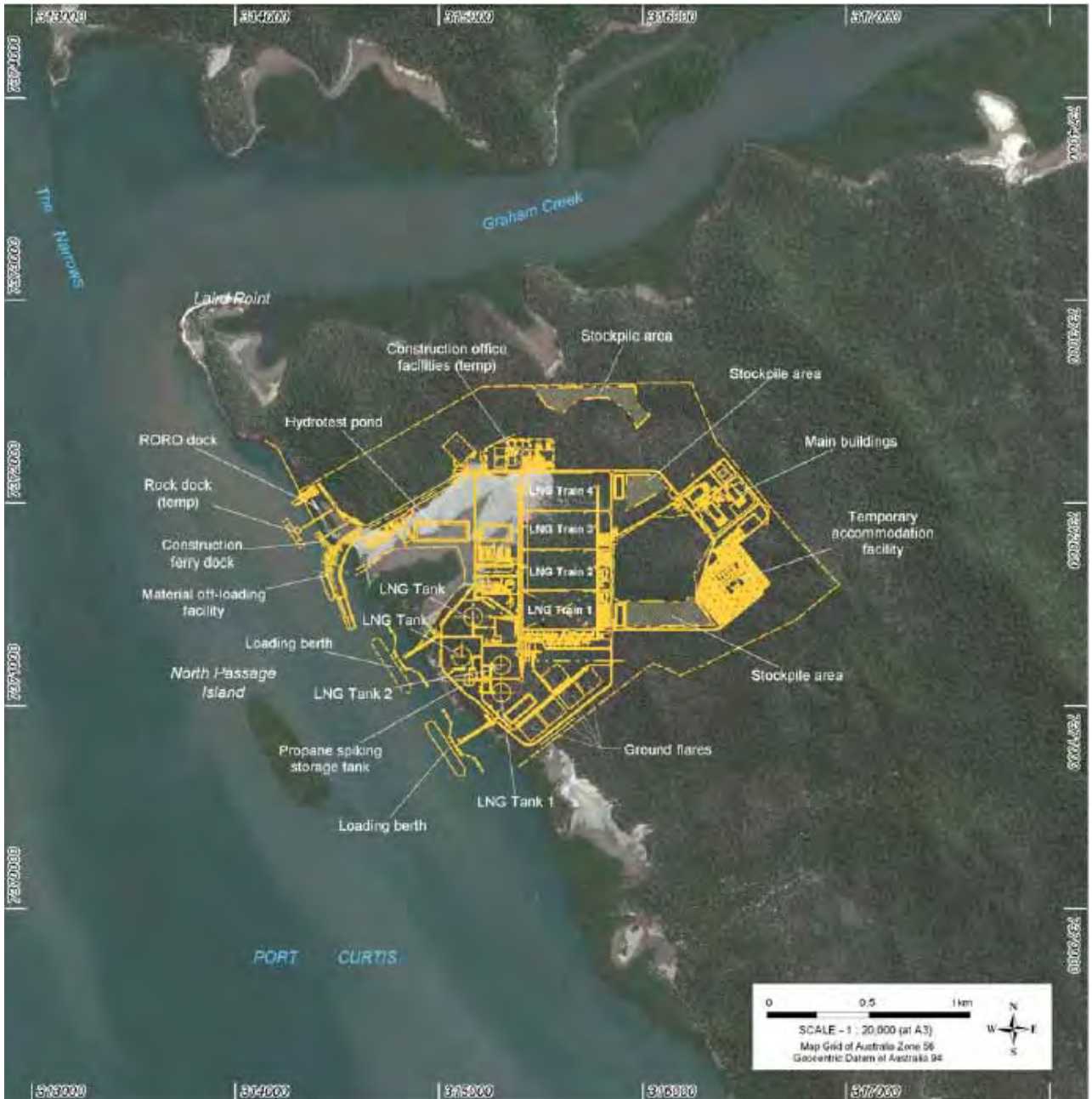
Figure 9.1—LNG facility layout
