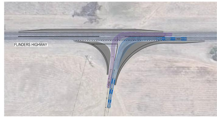
$\frac{26\text{m B-DOUBLE \& 8.8m SERVICE VEHICLE SWEPT PATH - INSET 1}}{\text{SCALE 1:500 (m)}}$
