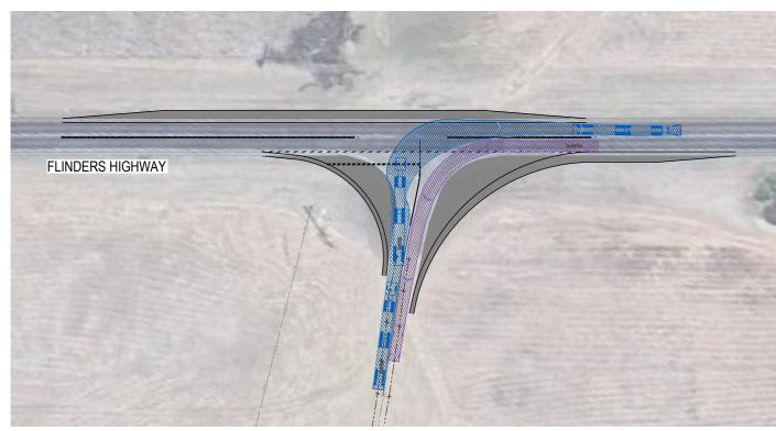
$\underbrace{26\text{m B-DOUBLE \& 8.8m SERVICE VEHICLE SWEPT PATH - INSET 2}}_{\text{SCALE 1:500 (m)}}$
