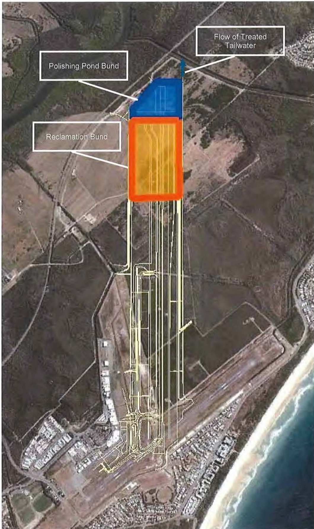
Figure 7.2 Revised Runway Design and Dredge Spoil Containment Area
