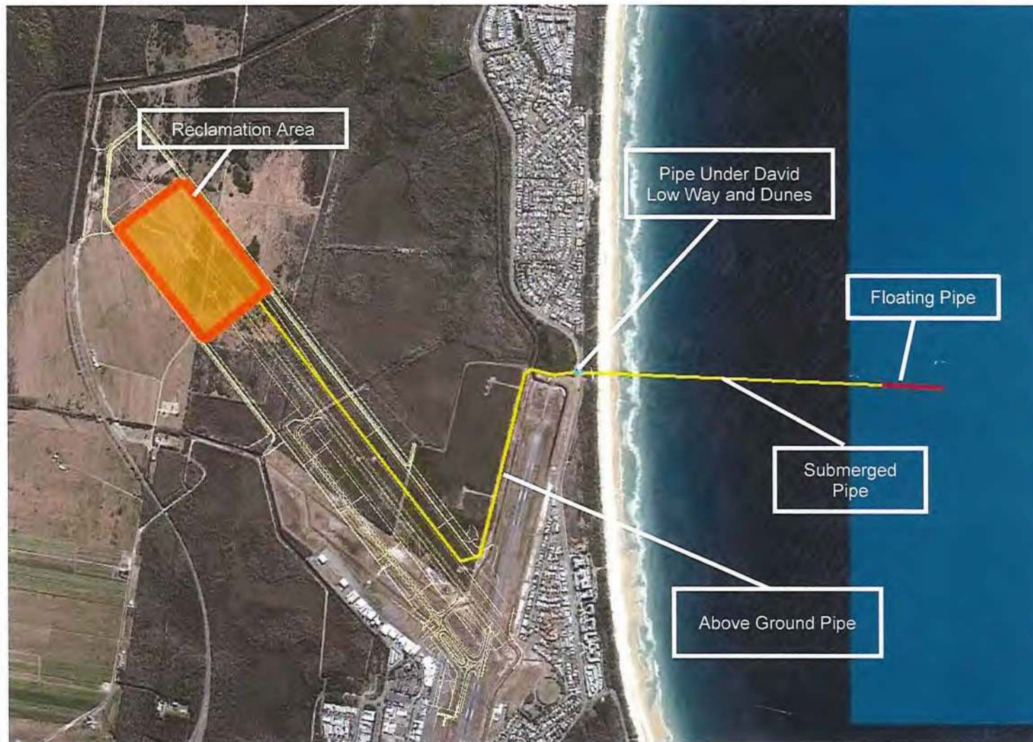
Figure 7.3 Revised Pipeline Alignment
