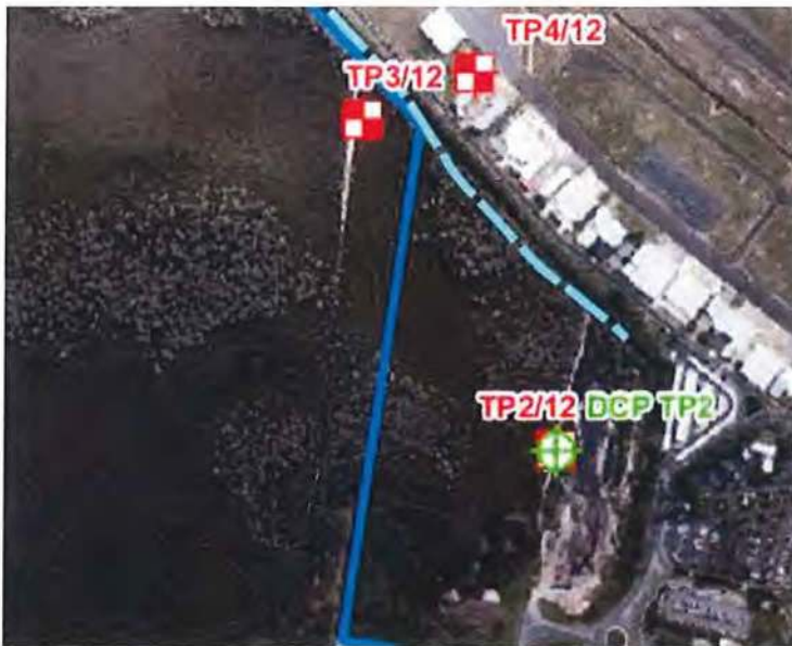
Map of Site showing all test pits in Mt Coolum National Park (Marcoola South Section) which soil salinity was measured.
