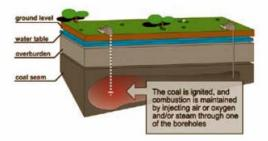
The coal is ignited at the bottom of the first well. Compressed air is introduced and this well becomes the injection well. The heat produced by the combustion of coal in the air and fuel-rich environment produces a combustible synthetic gas or syngas.
