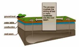
Two wells are drilled into the coal seam, typically at more than 100m (300 feet) deep and approximately 30m (90') apart. These wells are then joined inside the seam.
