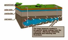
4. The gasification is carefully controlled, keeping the pressure inside the cavity below the groundwater hydrostatic pressure. This effectively provides a water seal around the reactor. Additional injection and production wells can be easily added, readily expanding the gasification front to increase gas production.
