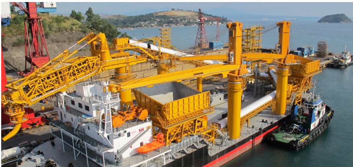
Photograph 2.6: Example of a transhipper (side view)
