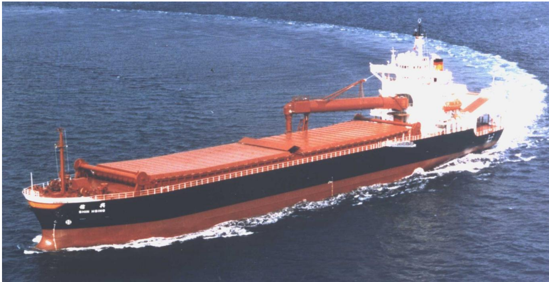
Photograph 2.4: Example of a self propelled, self unloading barge (SUB)
